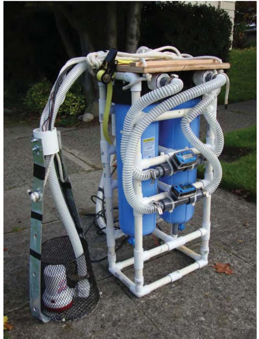
Figure 5. Suspended Solids Filtration Unit
