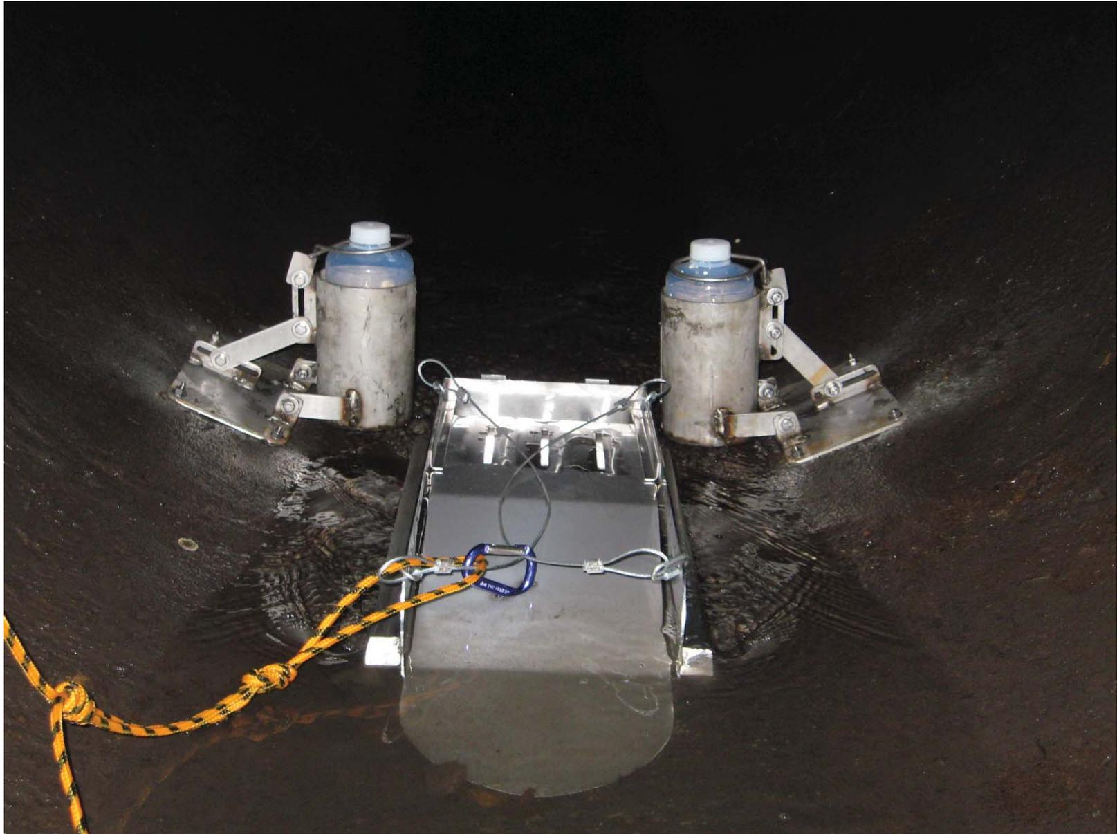
Figure 8. Ecology Bedload Sediment Trap
