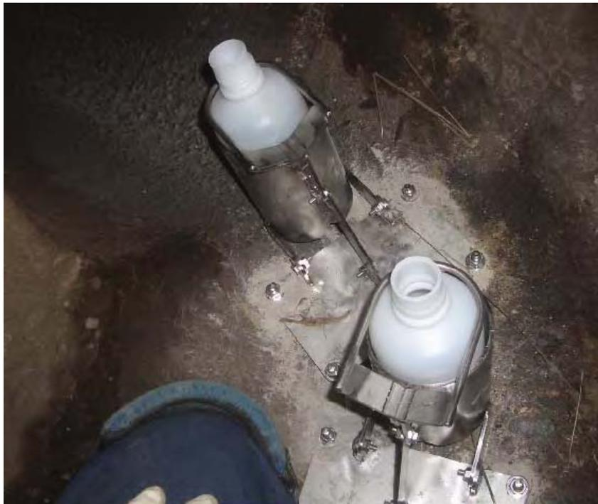
**Figure 7. Sediment Traps Installed
