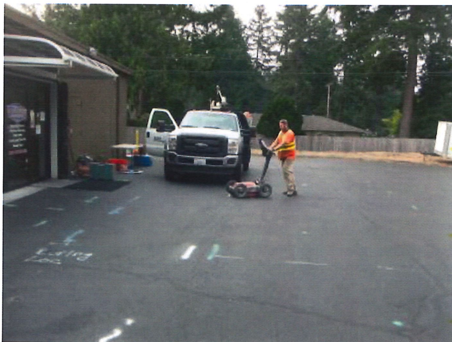
Photo 6. A view of the GPR survey.
