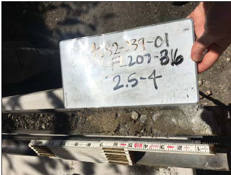
Photograph 4 – FL-207 – Boring location FL207-B16 showing soil core at 2.5 to 4 feet bgs. The sample from 2.5 to 3.5 feet bgs had a concentration of lube oil-range petroleum hydrocarbons greater than the MTCA Method A cleanup level.
