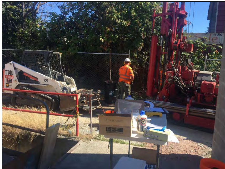
Photograph 6 – FL-207 – Boring location FL207-B18 south of loading dock. Soil from 0.5-1 foot bgs had a concentration of lube oil-range petroleum hydrocarbons greater than the MTCA Method A cleanup level.
