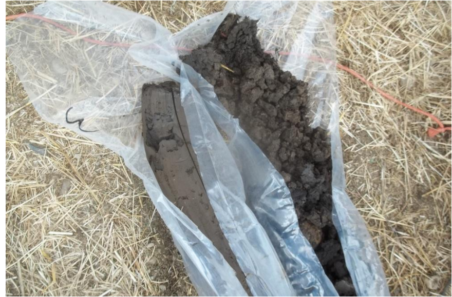
Typical recovered boring core consisted of areas of medium brown native soils.
