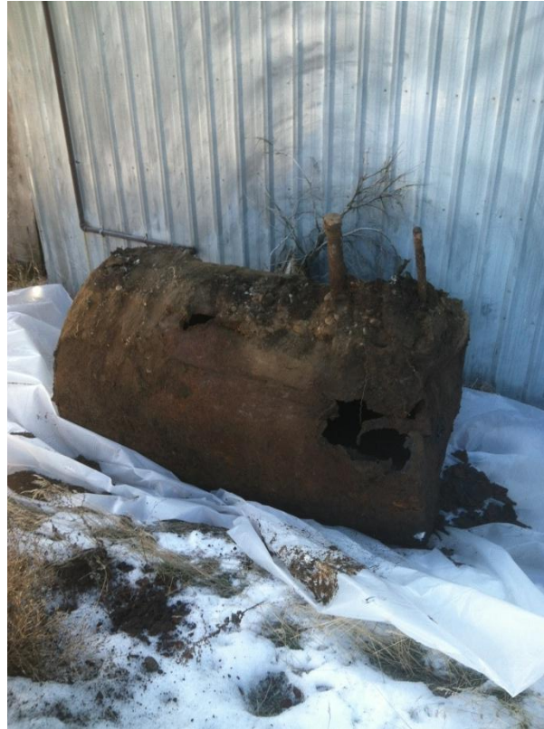
UST-04 following removal from site soils. Heavy corrosion was apparent.
