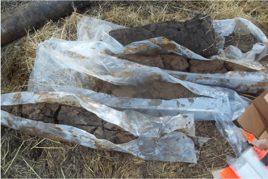
Recovered boring core in MW-02 including a layer of gray stained soil with a noticeable petroleum odor.
