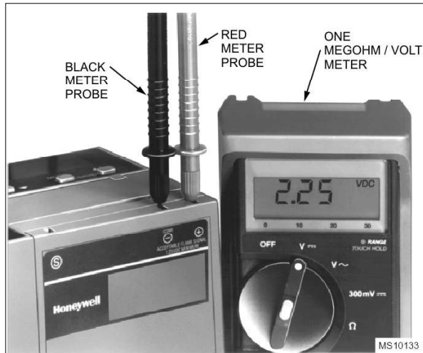
Fig. 11. Measuring voltage □ □ □ Signal with 7800 SERIES controls
