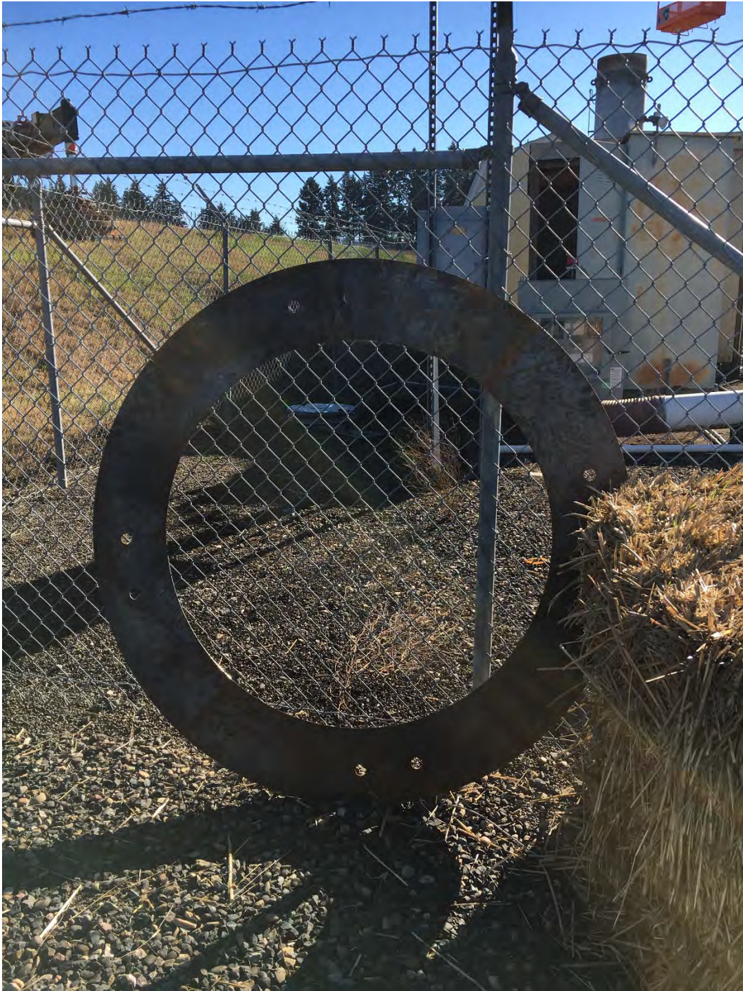
September 28, 2020 – Flare bolt alignment template for flare pad
