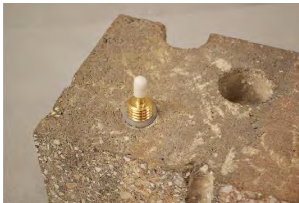
Figure 4. Installed Vapor Pin™.
