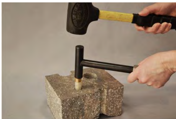
Figure 2. Installing the Vapor Pin™.
