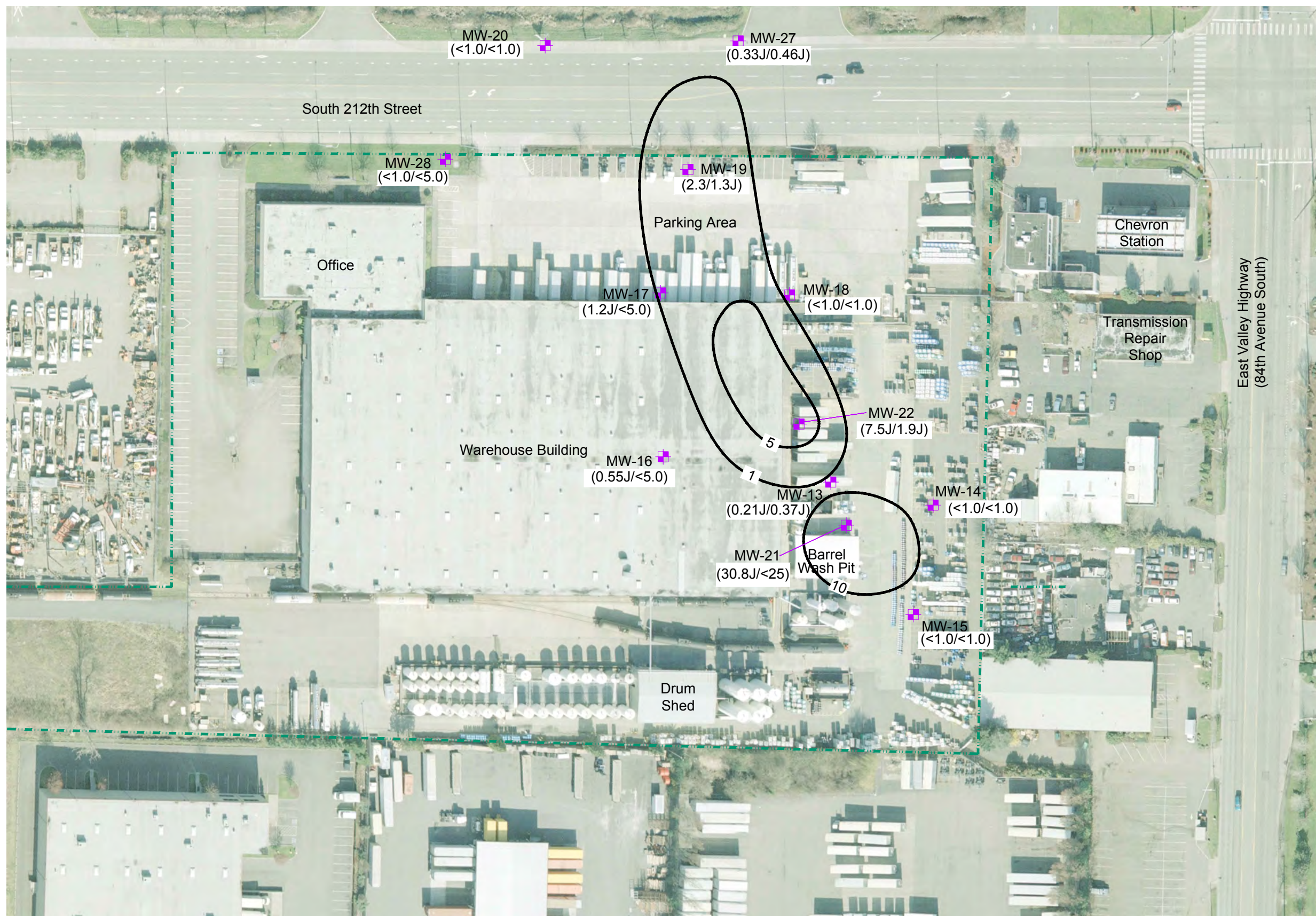
Figure 15 1,1-Dichloroethane Concentrations in Deep Groundwater
