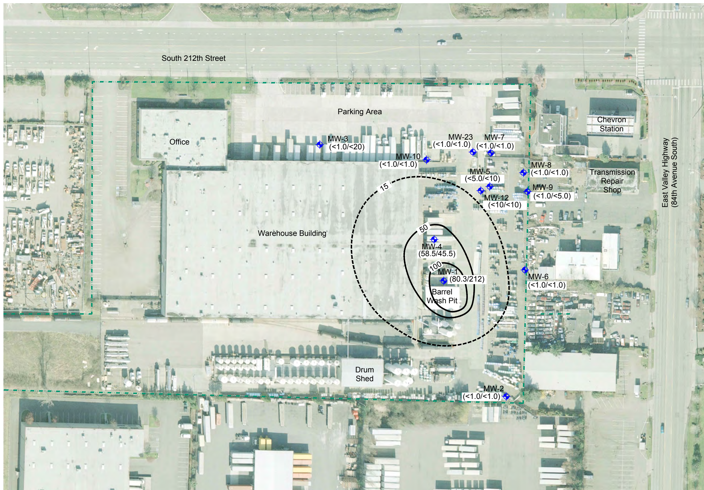
Figure 9 Chloroethane Concentrations in Shallow Groundwater
