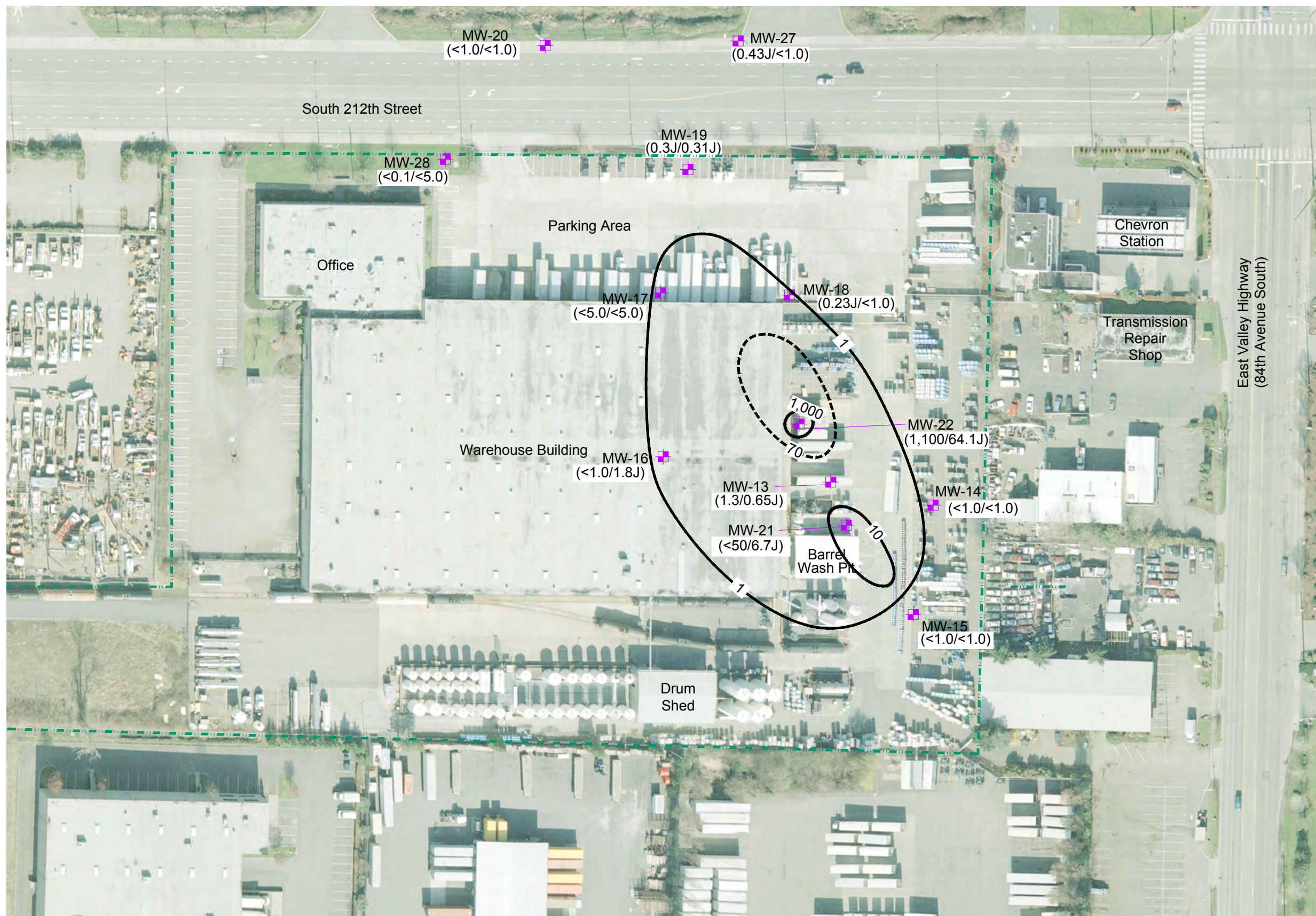
Figure 17 cis-1,2-Dichloroethene Concentrations in Deep Groundwater
