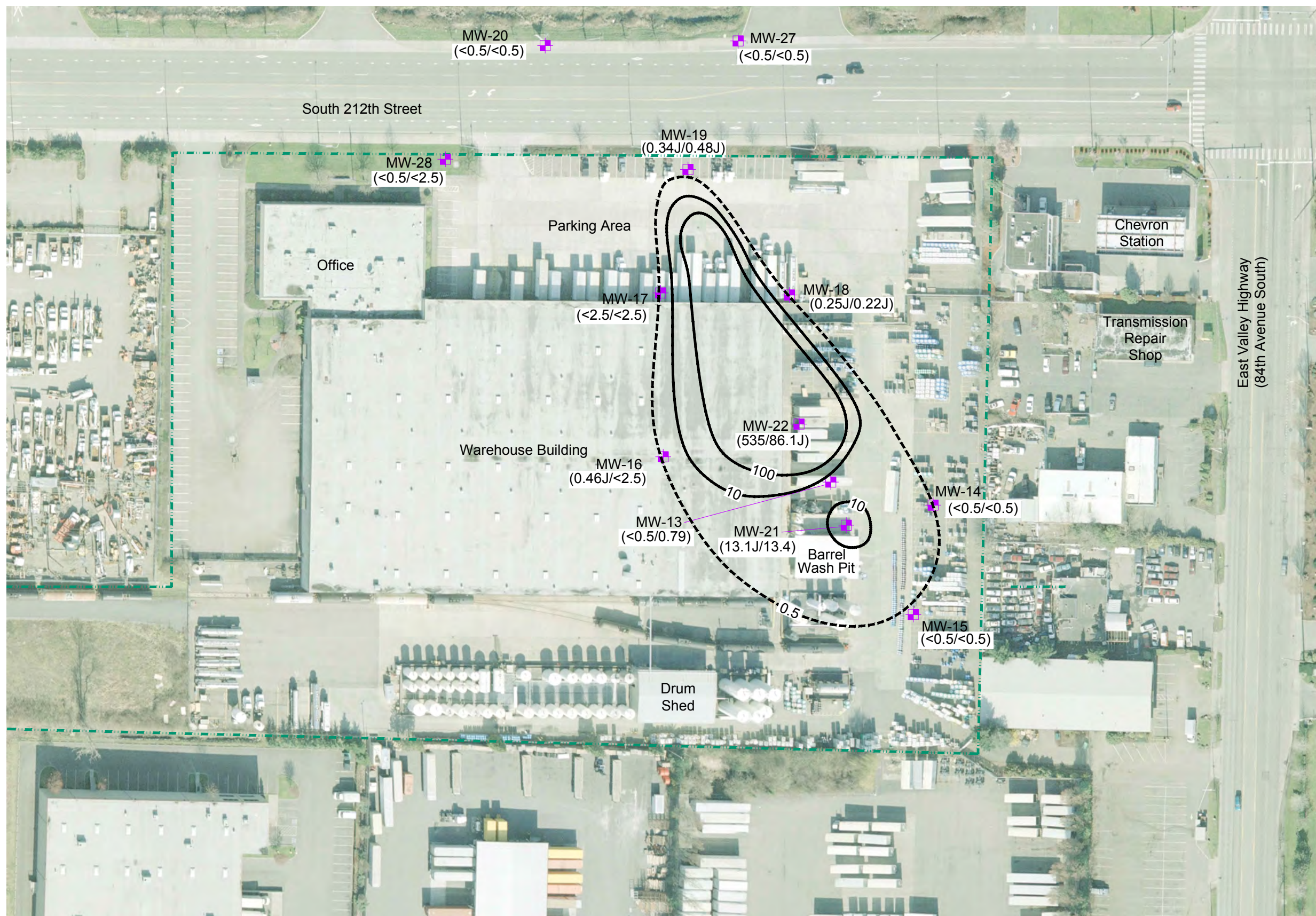
Figure 18 Vinyl Chloride Concentrations in Deep Groundwater
