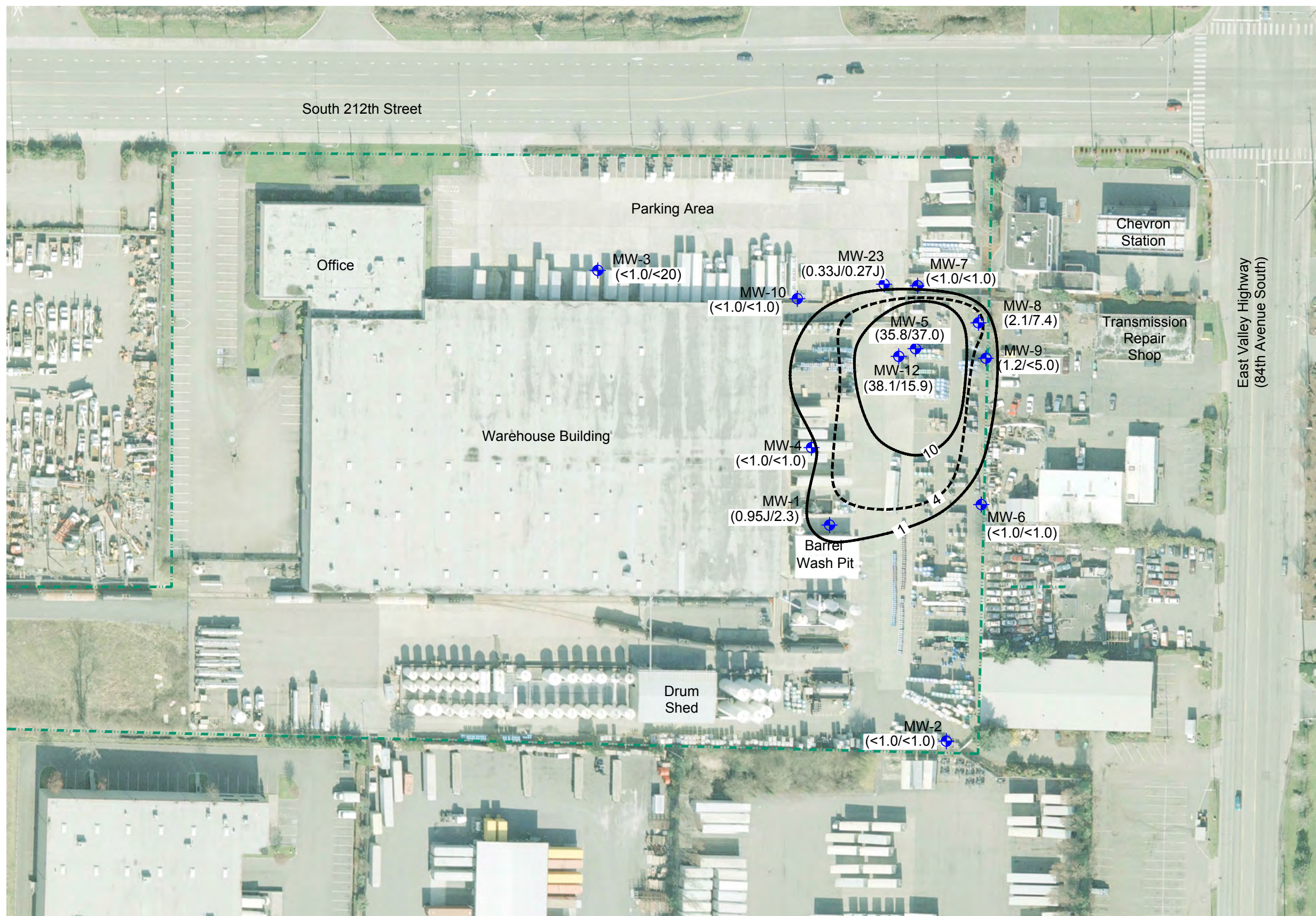
Figure 11 Trichloroethene Concentrations in Shallow Groundwater
