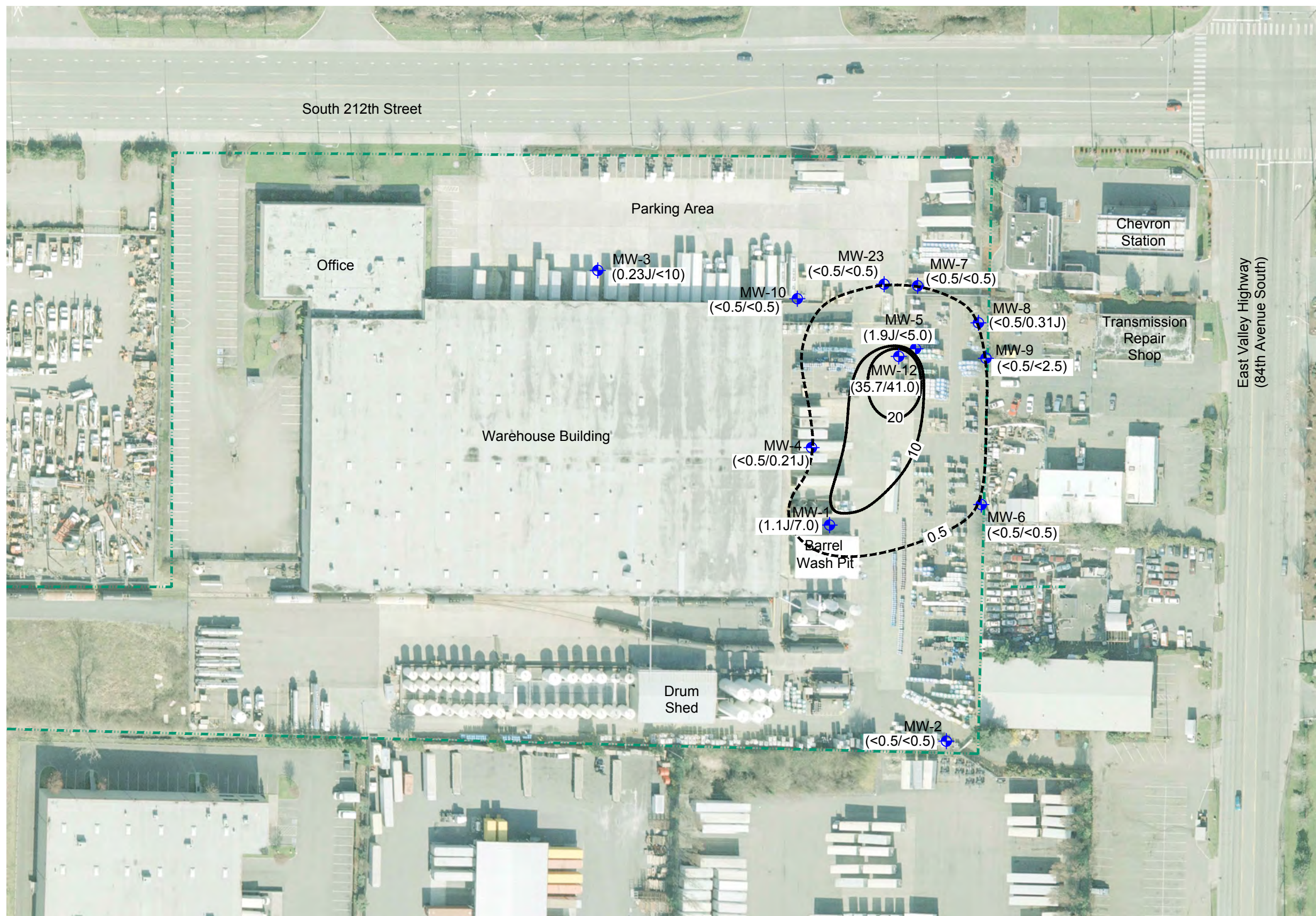
Figure 12 Vinyl Chloride Concentrations in Shallow Groundwater
