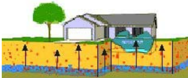
Solvents evaporating from groundwater and moving up through the soil. (Graphic courtesy of EnviroGroup Limited.)
