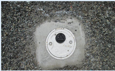
Figure 1. A monitoring well on the Boeing Auburn Site. Boeing will take samples from monitoring well access points to track the concentration of TCE on the Boeing Auburn site over time.
