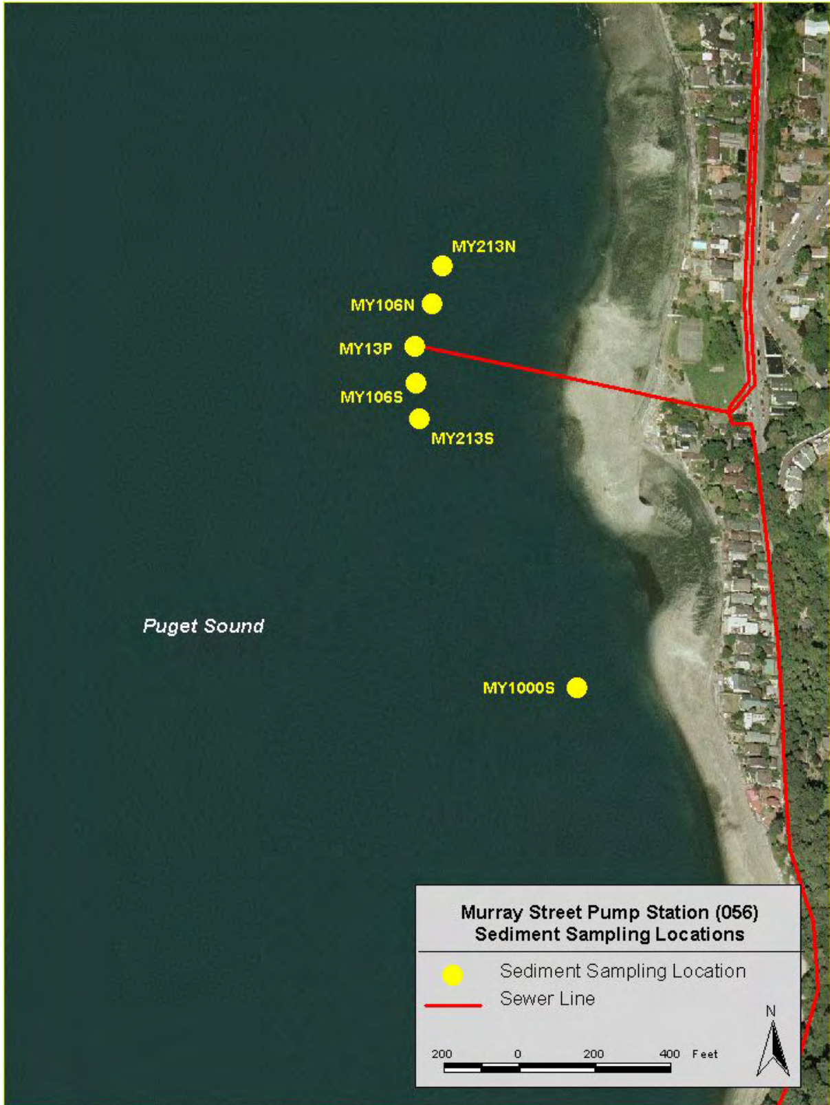
Figure 2-17. Murray Street Pump Station (056) Sediment Sampling Locations
