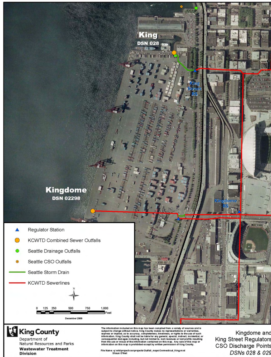
Figure 3-6. Connecticut Street (Kingdome) Regulator CSO Discharge Point
