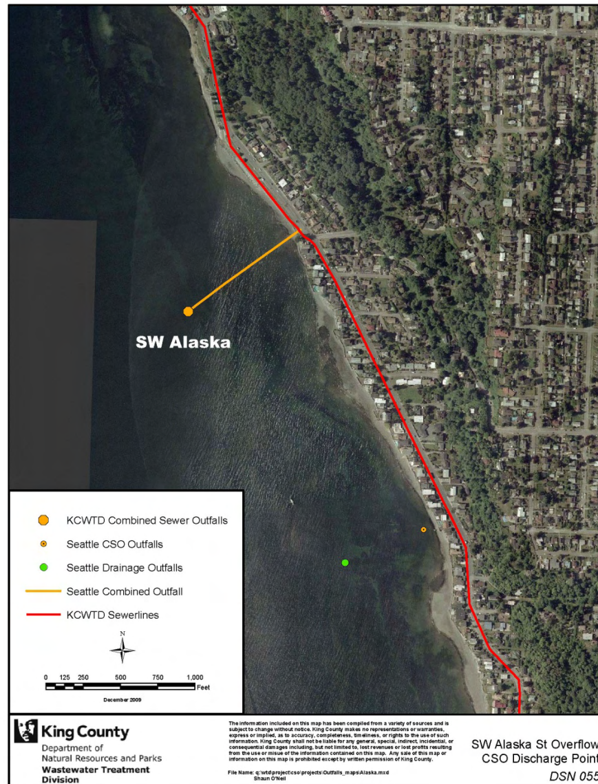
Figure 2-14. SW Alaska Street CSO Discharge Point
