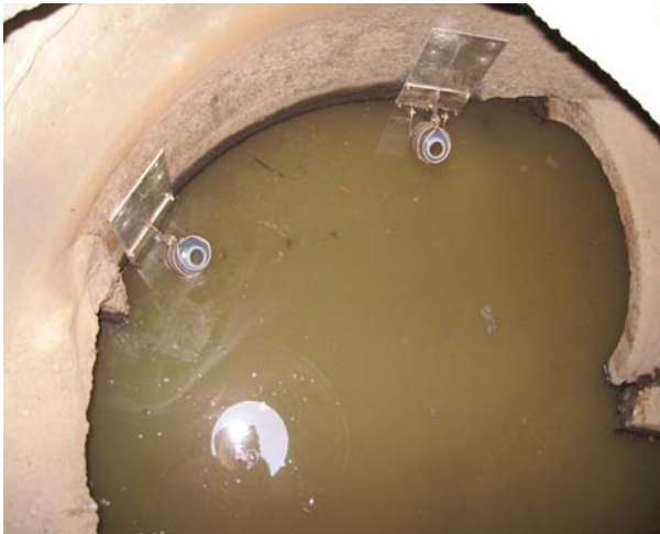
Figure 3: Sediment traps mounted vertically on the sidewall of a vault.
