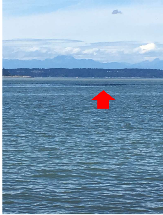
Photo 16: Looking North, location of submerged end of NPDES outfall is observable as a dark area on the water surface, which is due to the density difference between fresh and saltwater.
