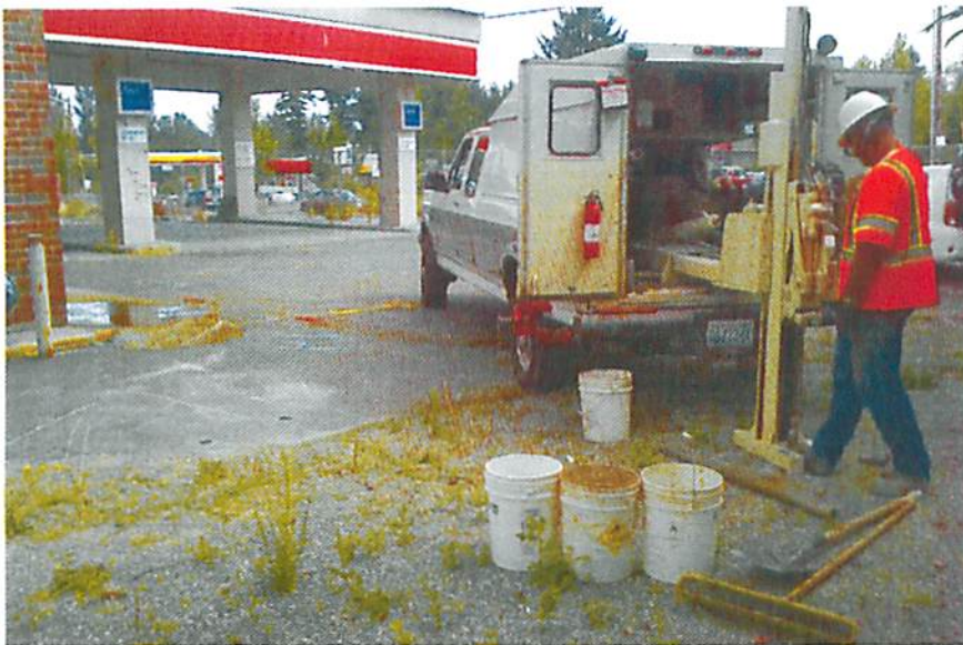
Borehole B-5 - Core tubes bottom to top: 4 ft, 8ft, 12ft, and 16ft - In situ diamiction at 15.3 to 16.0 ft (Beneath basin backfill)
