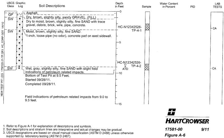
4. Groundwater conditions, if indicated, are at time of excavation. Conditions may vary with time.
