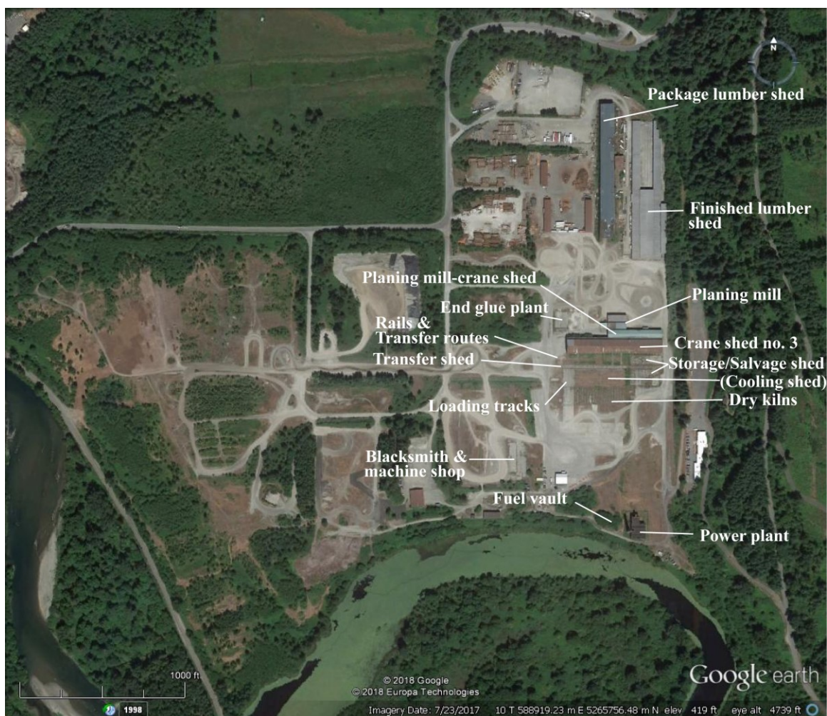
Figure 19. Buildings 40 years of age or older. The cooling shed is shown in parentheses because no physical remain was observed; the footprint of the former building is designated by distinctive vegetation.
