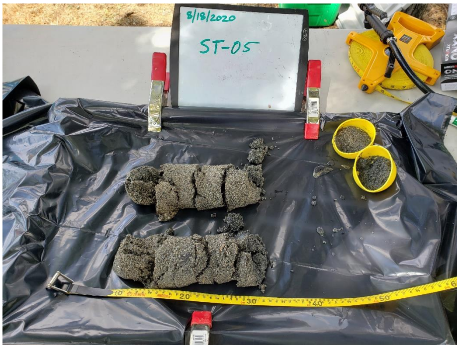
Photo 12: Sediment cores from Station ST-05 after extrusion from the core barrel
