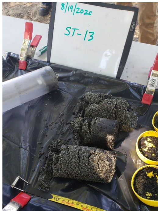
Photo 26: Sediment cores from Station ST-13 after extrusion from the core barrels
