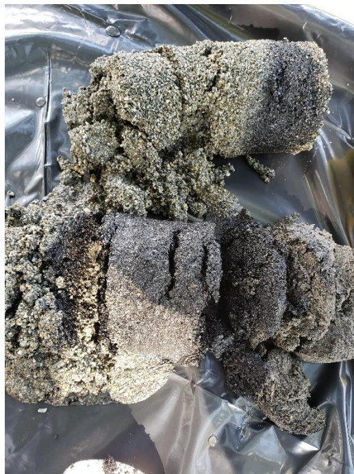
Photo 34: Sediment cores from Station ST-15 after extrusion from the core barrels
