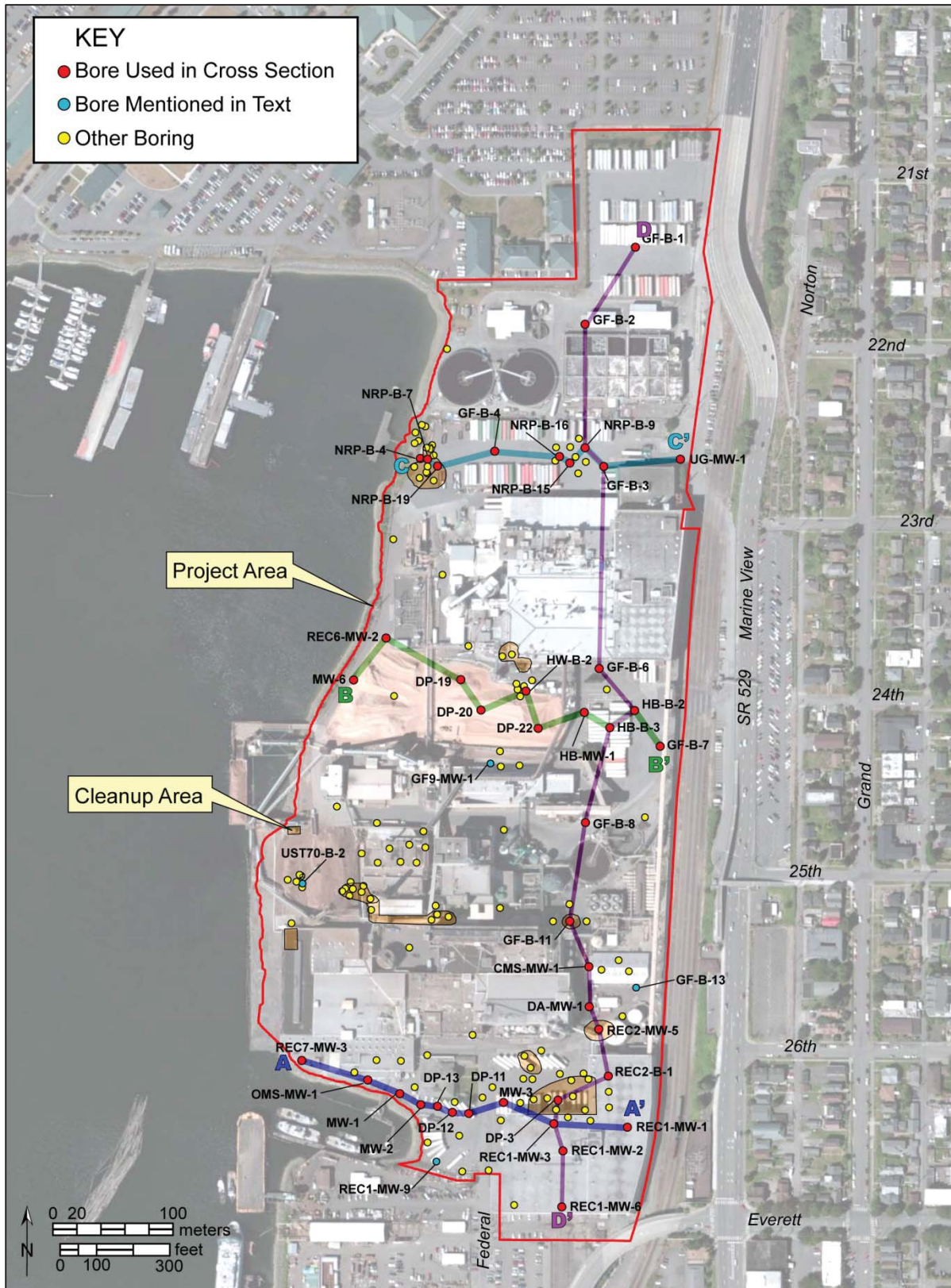
Figure 18. Map of previously completed borings used to model the sub-surface stratigraphy in the project area and cross-section transects in relation to opportunistic cleanup areas.
