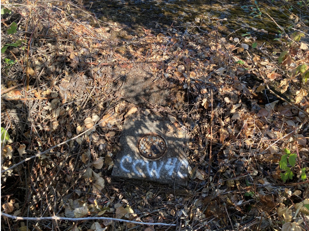
Picture 1 Monitoring Well CCW-4C on CleanCare Property
