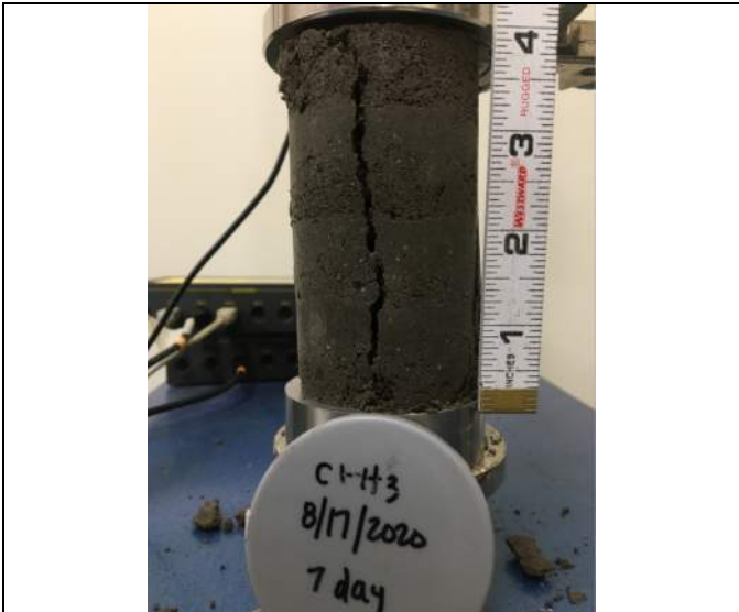
Picture Date: Monday 08/24/2020 Picture Taken By: Matt Polsky Picture Location: Chelmsford, Massachusetts Project Name: USG Highway 99 Site Project Description: C1-H3 UCS 7-day break
