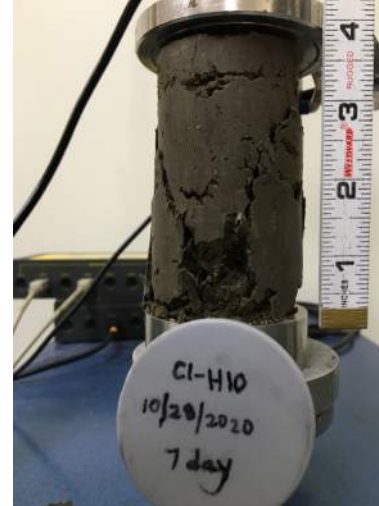
Picture Date: Wednesday 11/4/2020 Picture Taken By: Matt Polsky Picture Location: Chelmsford, Massachusetts Project Name: USG Highway 99 Site Project Description: C1-H10 UCS 7-day Break
