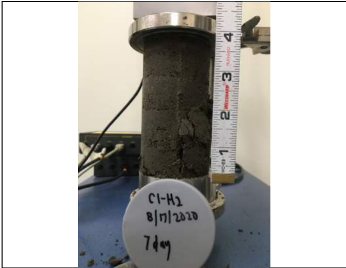
Picture Date: Monday 08/24/2020 Picture Taken By: Matt Polsky Picture Location: Chelmsford, Massachusetts Project Name: USG Highway 99 Site Project Description: C1-H2 UCS 7-day break
