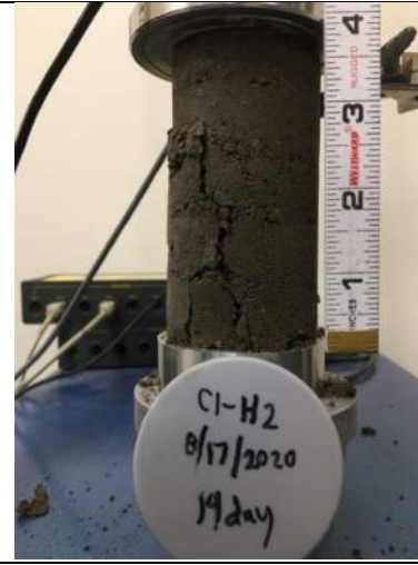
Picture Date: Monday 08/31/2020 Picture Taken By: Matt Polsky Picture Location: Chelmsford, Massachusetts Project Name: USG Highway 99 Site Project Description: C1-H2 UCS 14-day break
