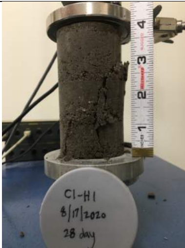
Picture Date: Monday 09/14/2020 Picture Taken By: Matt Polsky Picture Location: Chelmsford, Massachusetts Project Name: USG Highway 99 Site Project Description: C1-H1 UCS 28-day break
