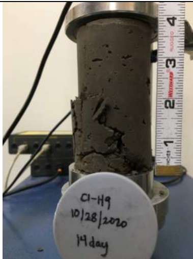
Picture Date: Wednesday 11/11/2020 Picture Taken By: Matt Polsky Picture Location: Chelmsford, Massachusetts Project Name: USG Highway 99 Site Project Description: C1-H9 UCS 14-day Break
