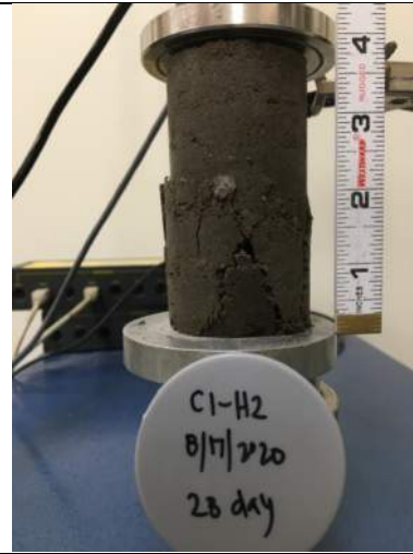
Picture Date: Monday 09/14/2020 Picture Taken By: Matt Polsky Picture Location: Chelmsford, Massachusetts Project Name: USG Highway 99 Site Project Description: C1-H2 UCS 28-day break
