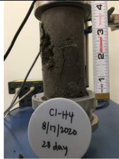
Picture Date: Monday 09/14/2020 Picture Taken By: Matt Polsky Picture Location: Chelmsford, Massachusetts Project Name: USG Highway 99 Site Project Description: C1-H4 UCS 28-day break
