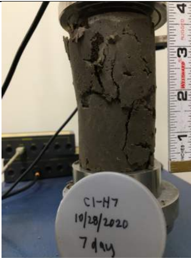
Picture Date: Wednesday 11/4/2020 Picture Taken By: Matt Polsky Picture Location: Chelmsford, Massachusetts Project Name: USG Highway 99 Site Project Description: C1-H7 UCS 7-day Break
