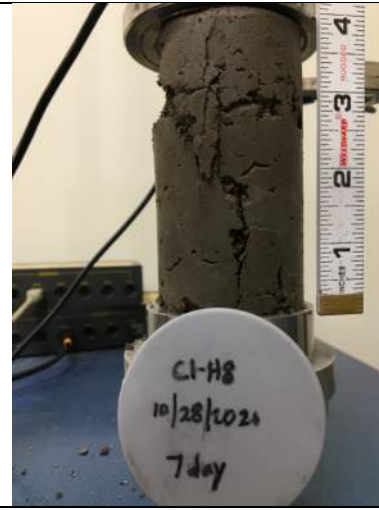
Picture Date: Wednesday 11/4/2020 Picture Taken By: Matt Polsky Picture Location: Chelmsford, Massachusetts Project Name: USG Highway 99 Site Project Description: C1-H8 UCS 7-day Break
