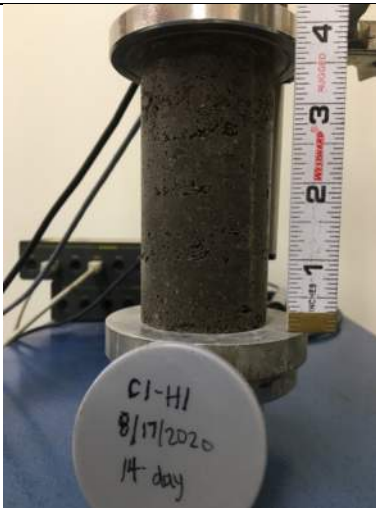
Picture Date: Monday 08/31/2020 Picture Taken By: Matt Polsky Picture Location: Chelmsford, Massachusetts Project Name: USG Highway 99 Site Project Description: C1-H1 UCS 14-day break
