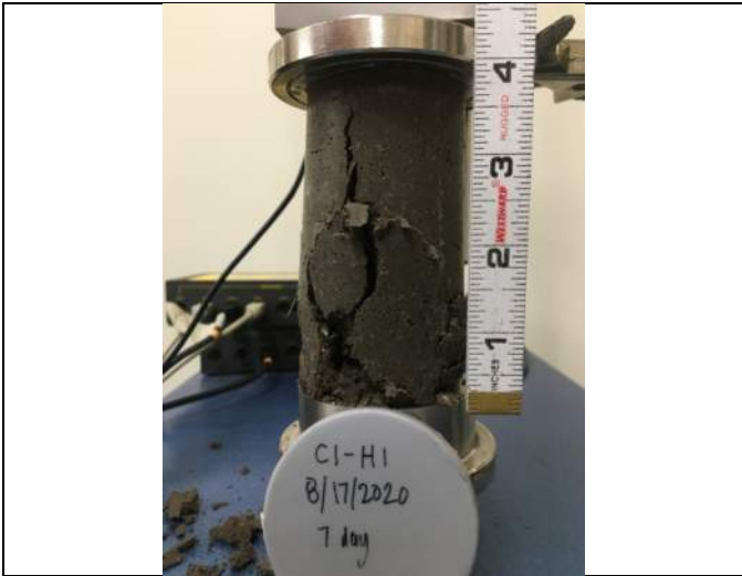
Picture Date: Monday 08/24/2020 Picture Taken By: Matt Polsky Picture Location: Chelmsford, Massachusetts Project Name: USG Highway 99 Site Project Description: C1-H1 UCS 7-day break
