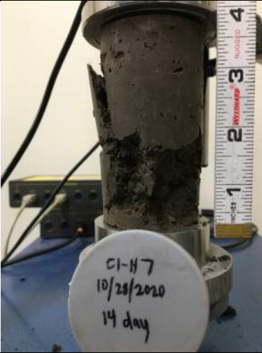
Picture Date: Wednesday 11/11/2020 Picture Taken By: Matt Polsky Picture Location: Chelmsford, Massachusetts Project Name: USG Highway 99 Site Project Description: C1-H7 UCS 14-day Break
