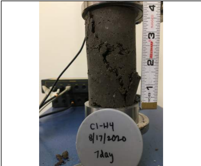
Picture Date: Monday 08/24/2020 Picture Taken By: Matt Polsky Picture Location: Chelmsford, Massachusetts Project Name: USG Highway 99 Site Project Description: C1-H4 UCS 7-day break
