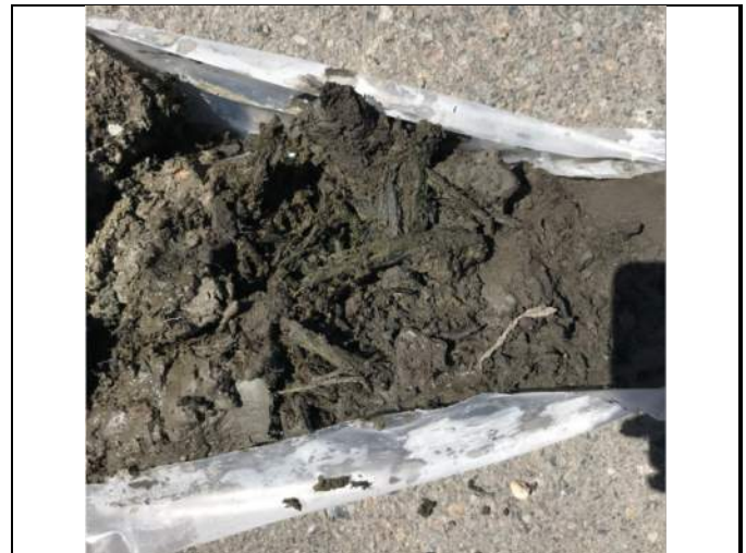
Picture Date: Friday 08/7/2020 Picture Taken By: Haley Provinsal Picture Location: Milton, Washington Project Name: USG Highway 99 Site Description: 99-BS-1, C-4 wood debris
