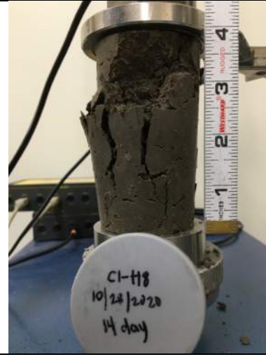
Picture Date: Wednesday 11/11/2020 Picture Taken By: Matt Polsky Picture Location: Chelmsford, Massachusetts Project Name: USG Highway 99 Site Project Description: C1-H8 UCS 14-day Break
