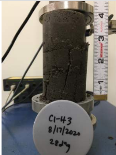
Picture Date: Monday 09/14/2020 Picture Taken By: Matt Polsky Picture Location: Chelmsford, Massachusetts Project Name: USG Highway 99 Site Project Description: C1-H3 UCS 28-day break
