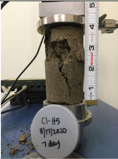
Picture Date: Monday 08/24/2020 Picture Taken By: Matt Polsky Picture Location: Chelmsford, Massachusetts Project Name: USG Highway 99 Site Project Description: C1-H5 UCS 7-day break
