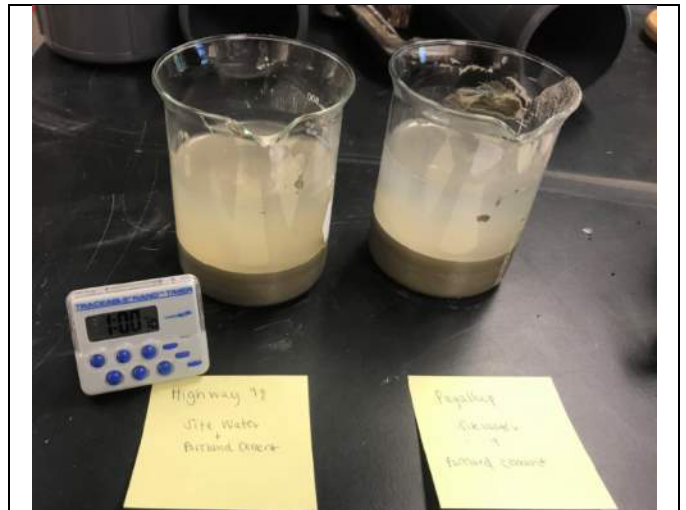
Picture Date: Tuesday 08/11/2020 Picture Taken By: Haley Provinsal Picture Location: Bellevue, Washington Project Name: USG Highway 99/Puyallup Sites Project Description: Time Passed = 1 hour Portland Cement and site water
