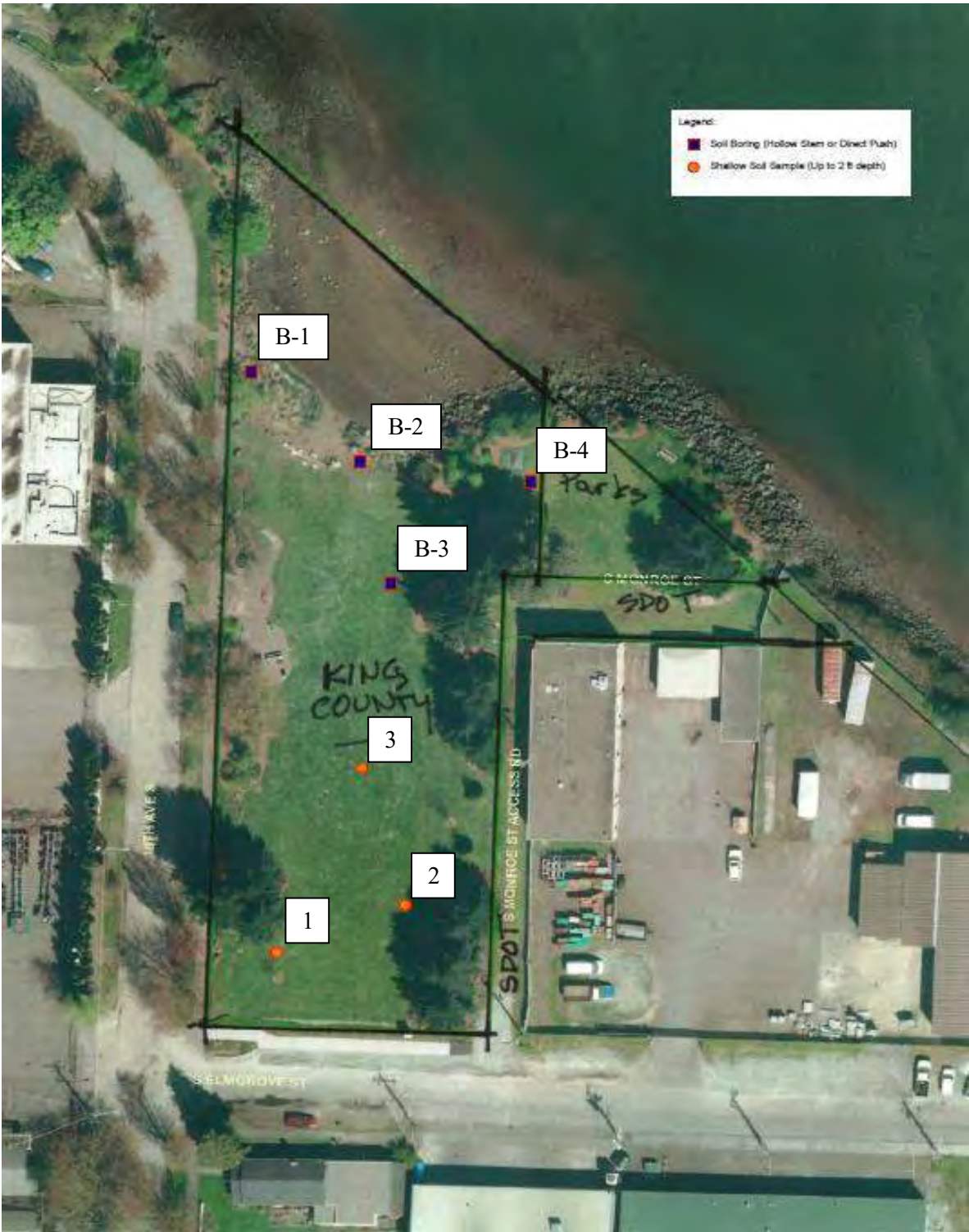
Figure 1. Approximate soil sampling locations. Duwamish Waterway Park. January 18, 2019.
