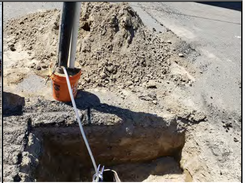
Infiltration test setup at P-4
