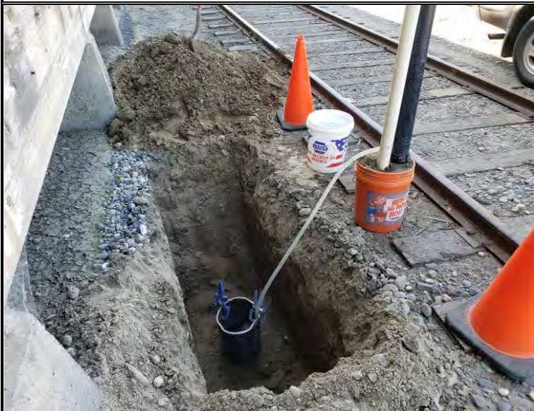
Infiltration test setup at P-5
