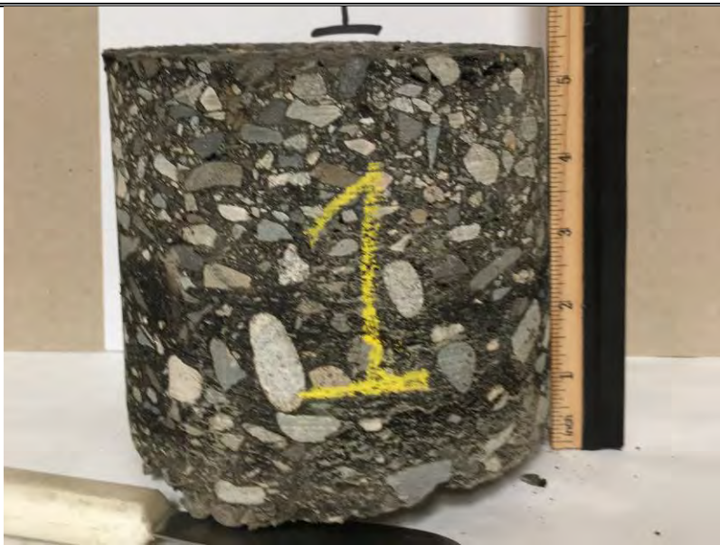
Pavement core sample obtained from Core #1
