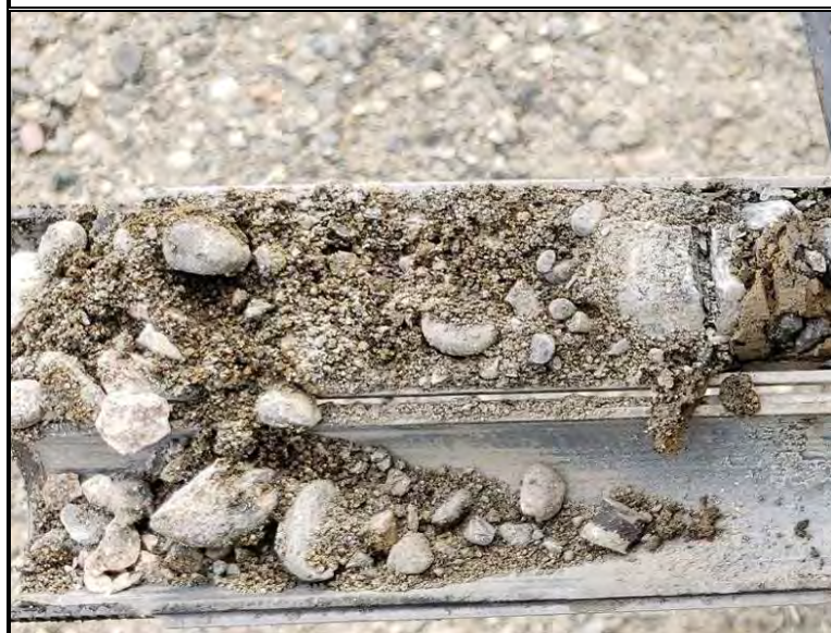
Split-spoon sample obtained from borehole B-9 @ 5' BGS
