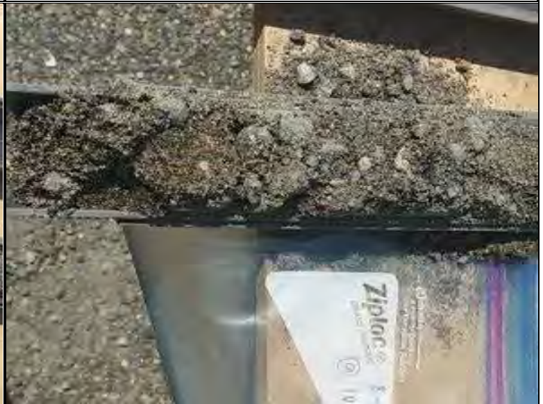
Split-spoon sample obtained from borehole B-15 @ 10' BGS
