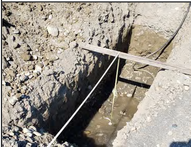
Infiltration test setup at P-1
