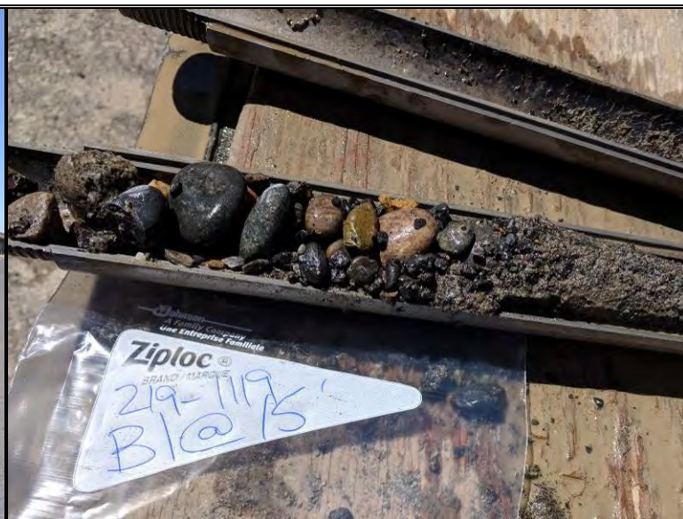
Split-spoon sample obtained from borehole B-1 @ 15' BGS
