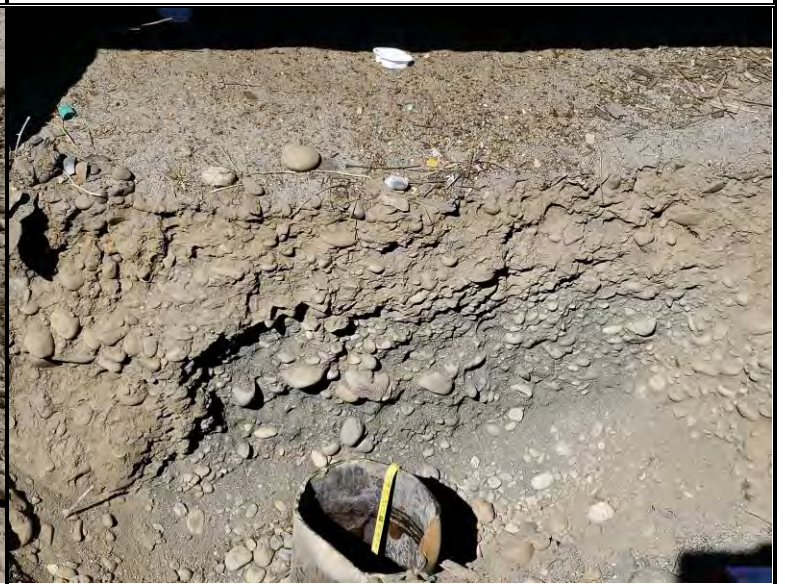
Infiltration test setup at P-17
