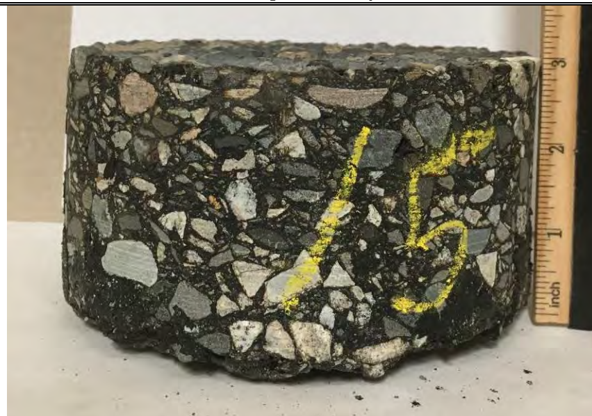
Pavement core sample obtained from Core #15
