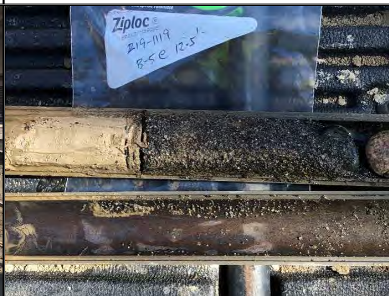
Split-spoon sample obtained from borehole B-5 @ 12.5' BGS
