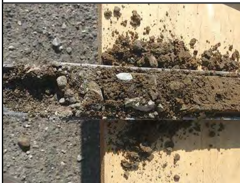
Split-spoon sample obtained from borehole B-10 @ 5' BGS
