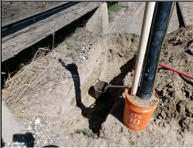
Infiltration test setup at P-12
