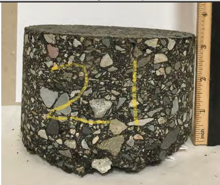
Pavement core sample obtained from Core #21
