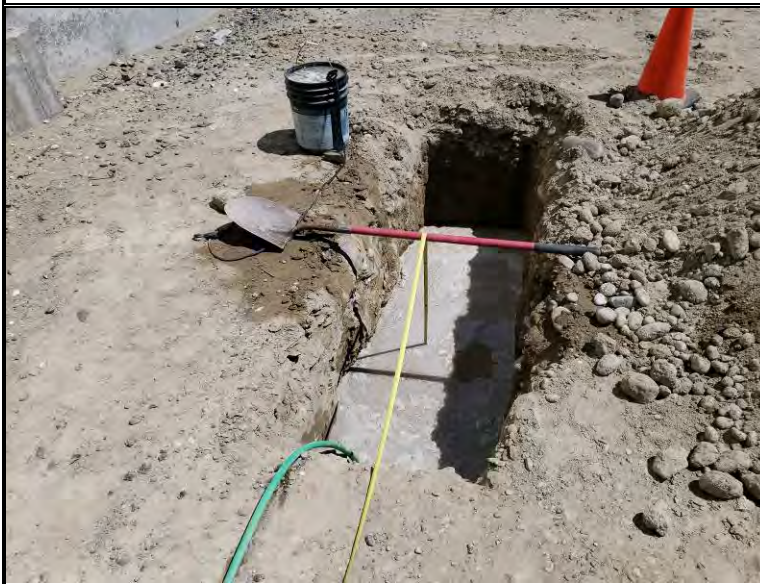
Infiltration test setup at P-16
