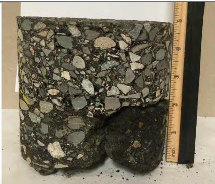
Pavement core sample obtained from Core #19
