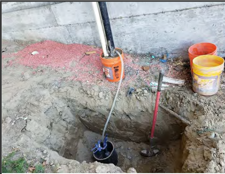
Infiltration test setup at P-3
