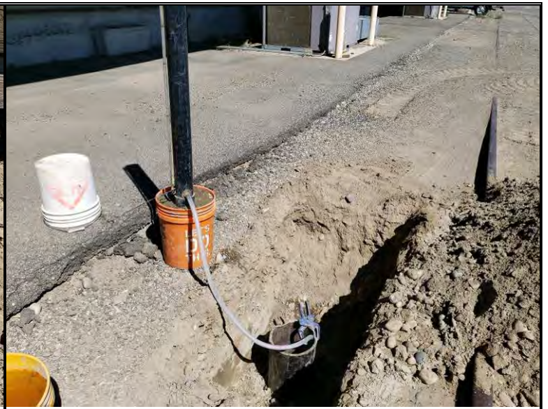
Infiltration test setup at P-11
