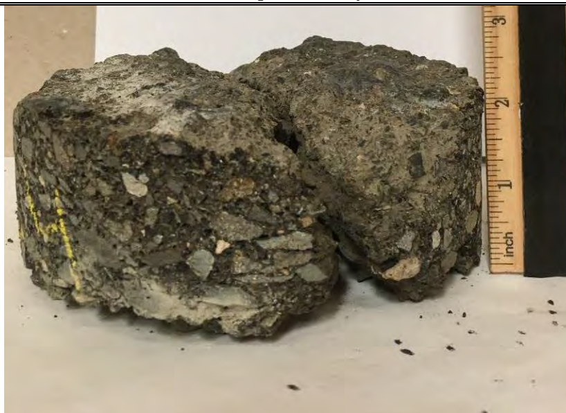
Pavement core sample obtained from Core #24
