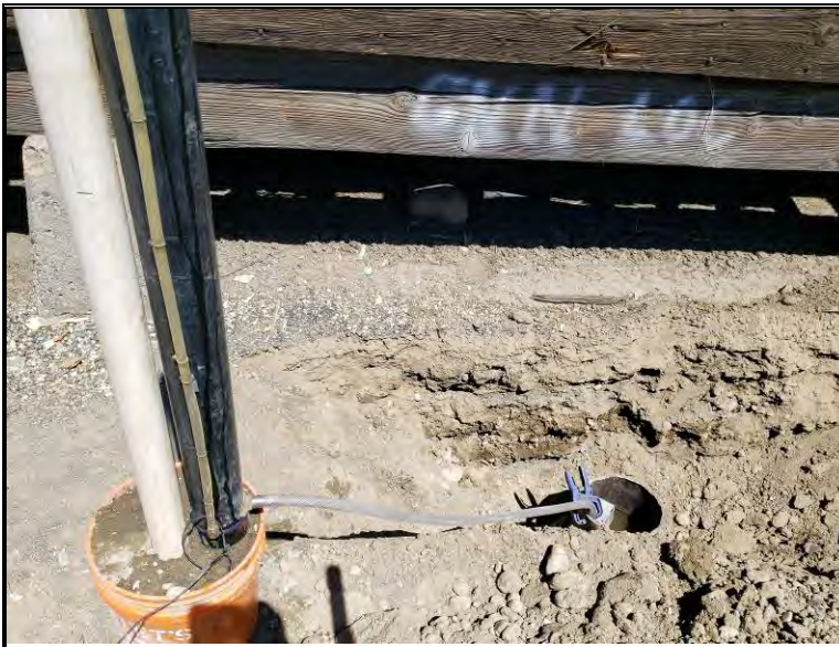
Infiltration test setup at P-9
