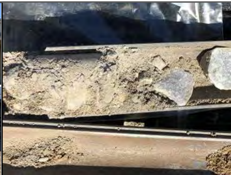
Split-spoon sample obtained from borehole B-6 @ 5' BGS
