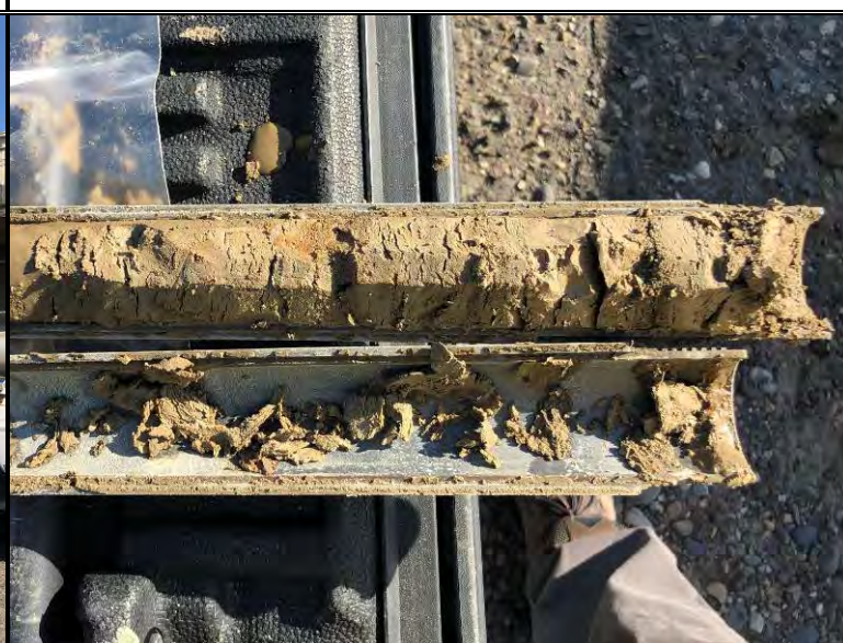
Split-spoon sample obtained from borehole B-4 @ 10' BGS
