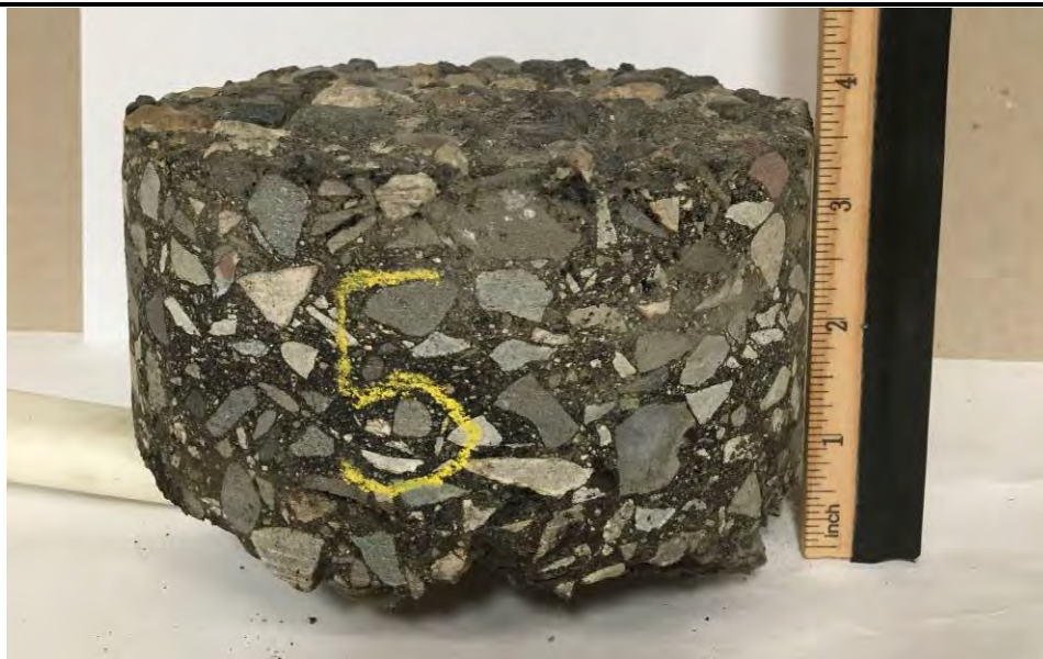
Pavement core sample obtained from Core #5
