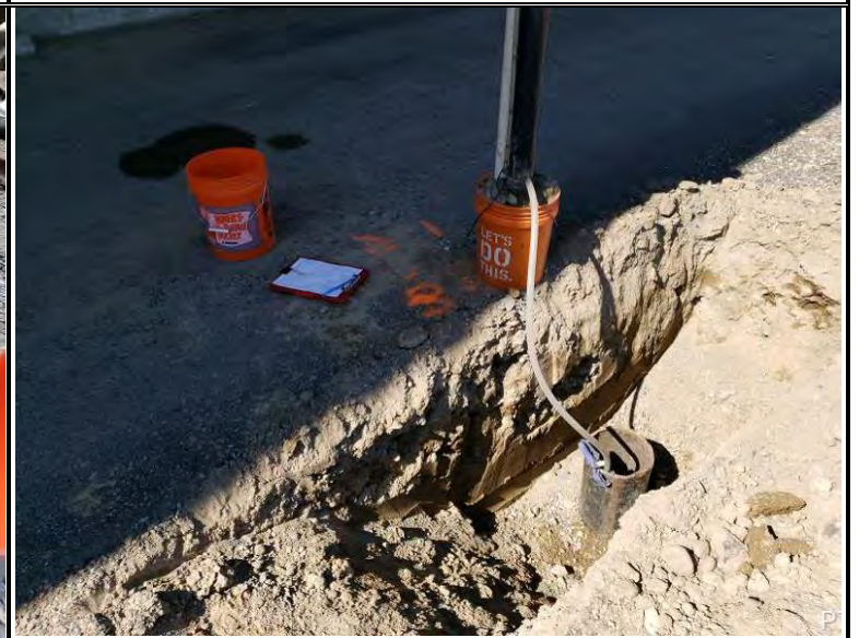
Infiltration test setup at P-7
