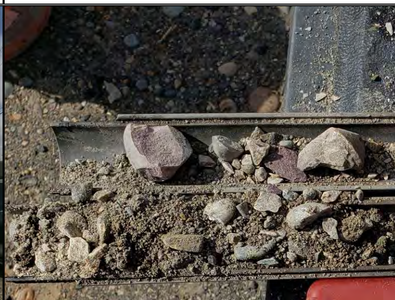
Split-spoon sample obtained from borehole B-8 @ 10' BGS
