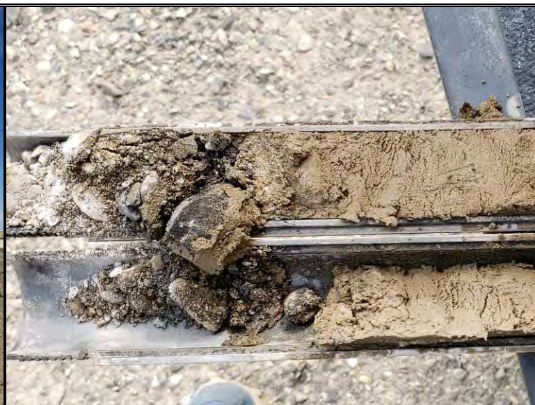
Split-spoon sample obtained from borehole B-9 @ 2.5' BGS
