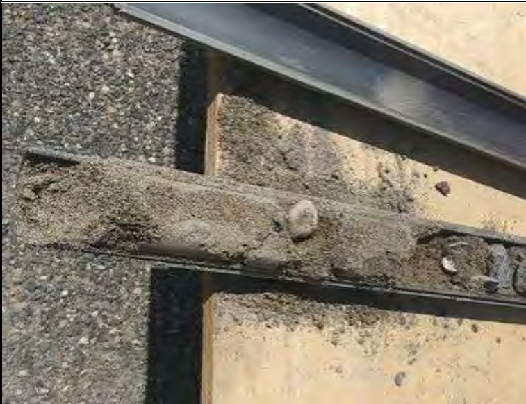
Split-spoon sample obtained from borehole B-14 @ 5' BGS
