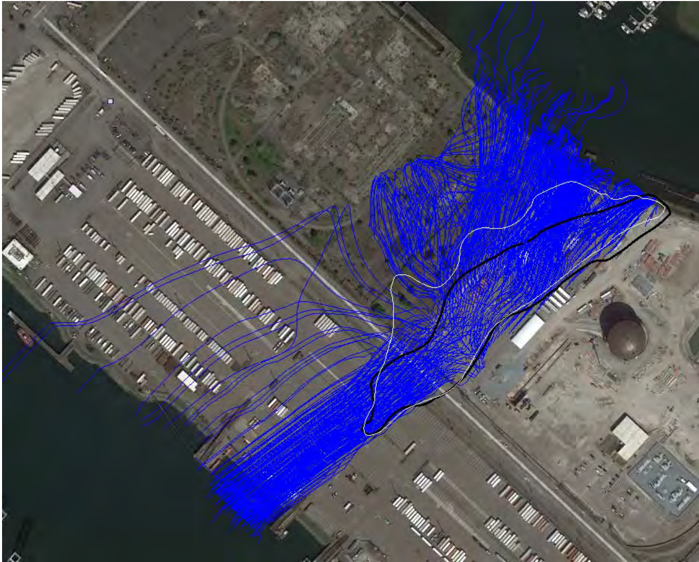
Figure 2. Particle tracks for benzene in the shallow aquifer with the “No Action” alternative. Concentration information provided by C. San Juan, Ecology. Plume contour shown in black corresponds to 24 ug/L benzene and and contours shown in white corresponds to 800 ug/L GRO. Blue tracks discharge to Hylebos Waterway.
