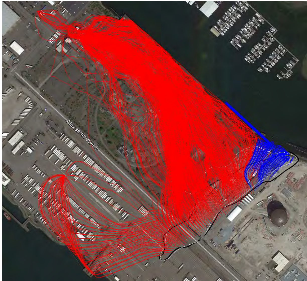
Figure 1. Particle tracks for benzene in the shallow aquifer with the “MSP” pumping system. Concentration information provided by C. San Juan, Ecology. Plume contour shown in black corresponds to 24 ug/L benzene and and contours shown in white corresponds to 800 ug/L GRO. Blue tracks discharge to Hylebos Waterway; red tracks are captured by pumping system.
