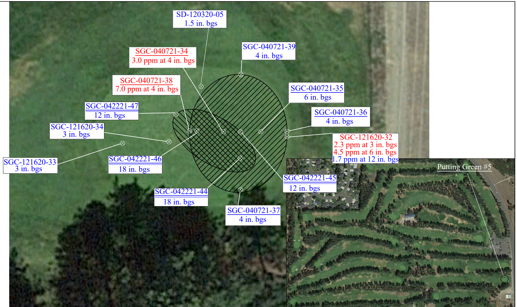
Figure 5: Putting Green #5 - Remedial Excavation and Characterization/Confirmatory Soil Sample Locations for Mercury Contaminated Soil
