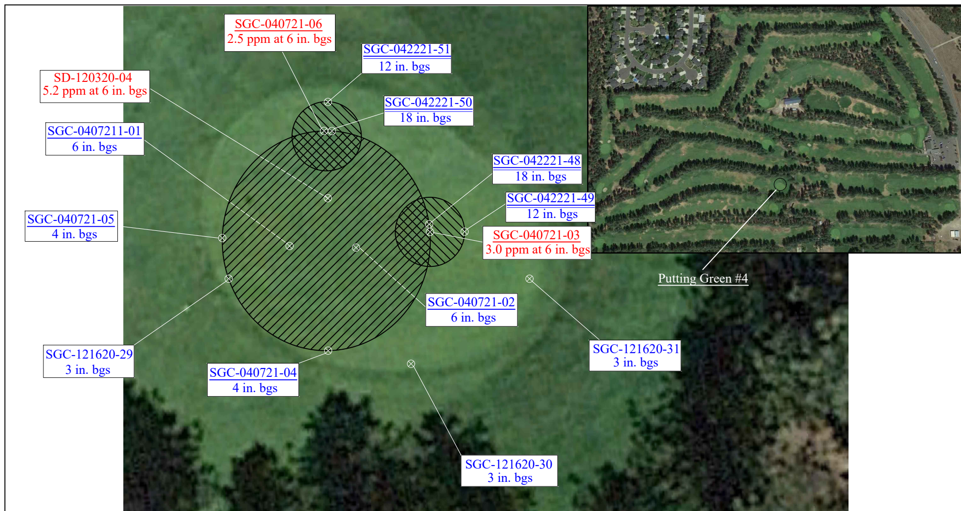
Figure 4: Putting Green #4 - Remedial Excavation and Characterization/Confirmatory Soil Sample Locations for Mercury Contaminated Soil
