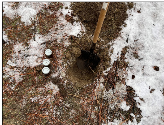
View of typical near-surface mercury characterization sample location completed throughout the subject site.
