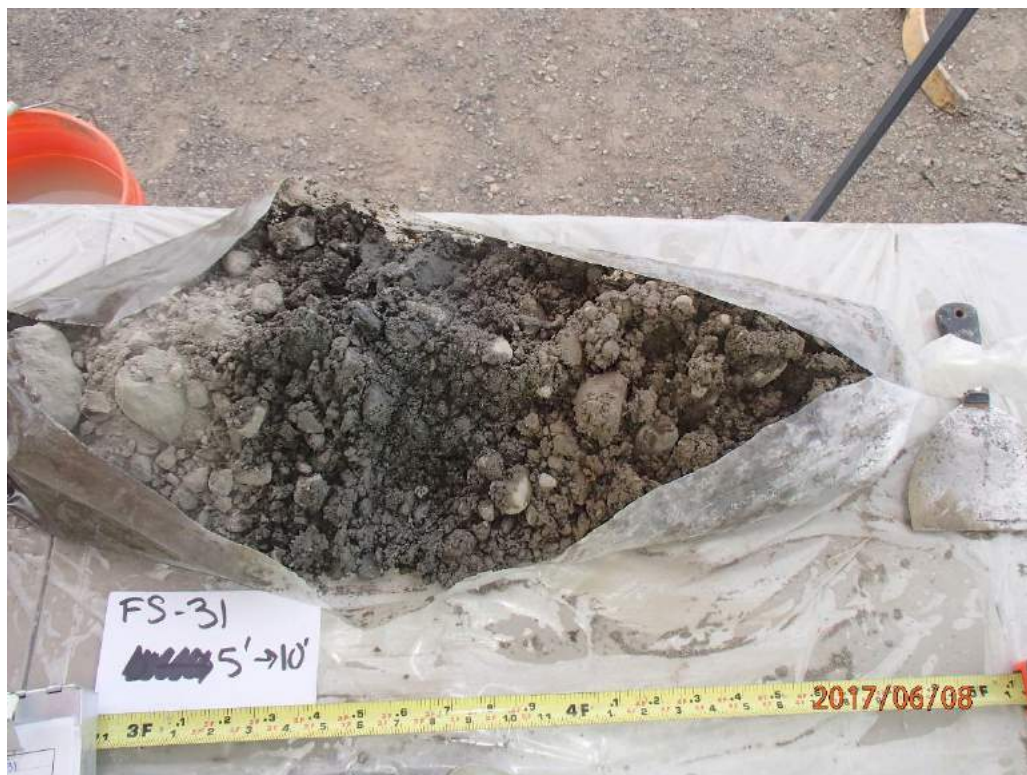
Photograph 20. Soil recovered from boring FS-31 showing petroleum-impacted interval collected during RI Phase 2A. June 2017.
