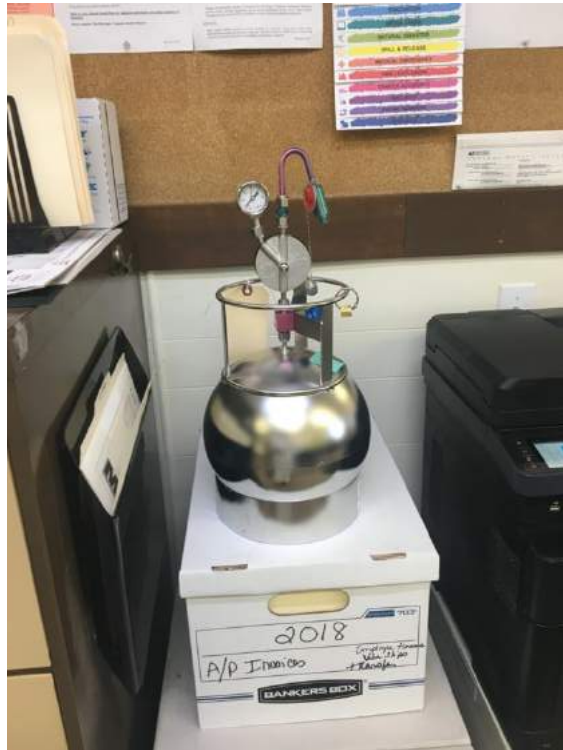
Photograph 3. Indoor air SUMMA canister; approximately 4 feet above ground and adjacent to copier.
