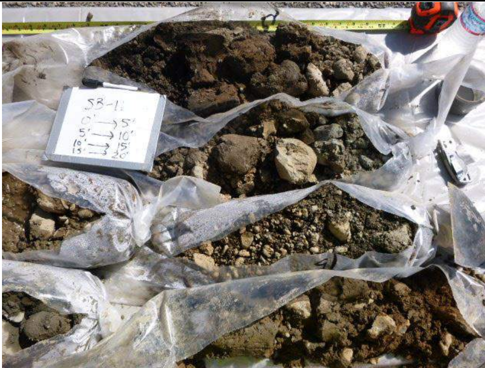
Photograph 15. Soil representative of subsurface conditions at Smith-Kem site (organic-rich silt/silty gravel above well-graded gravel and silty gravels) recovered from FS-11 during RI Phase 1. August 2016.
