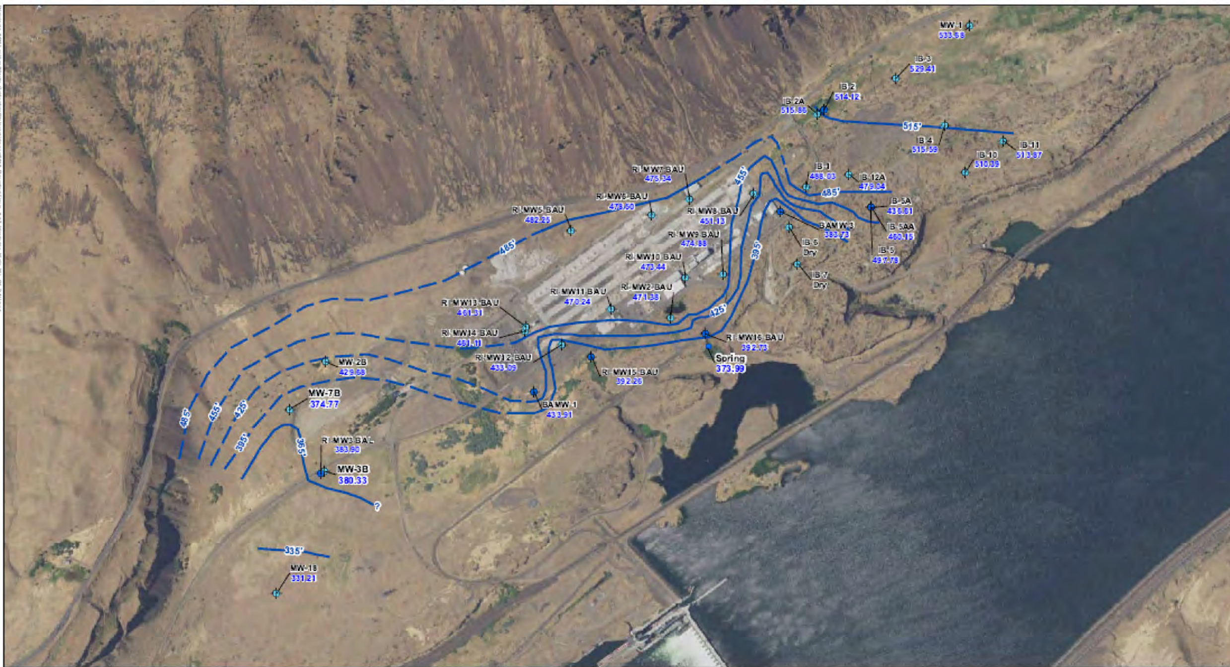
Figure 2-17 Water-Level Elevations Uppermost Basalt Aquifer Wells (BAU) Quarter 1 (Winter 2017)
