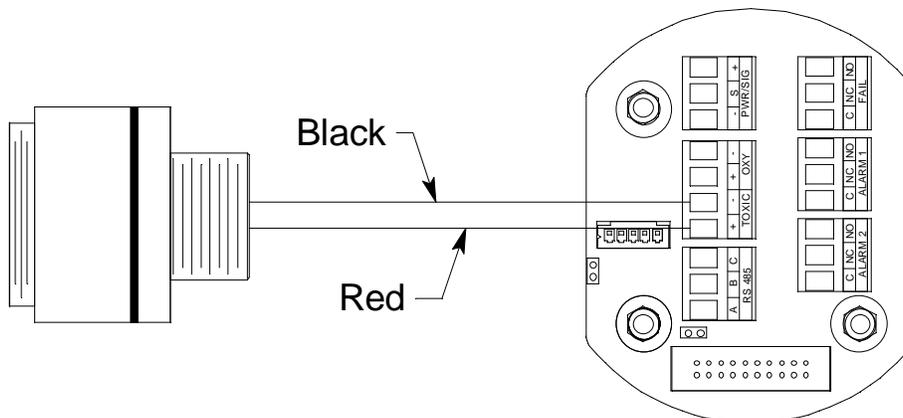
**Figure 24: H<sub>2</sub>S/CO Detector Wiring**
