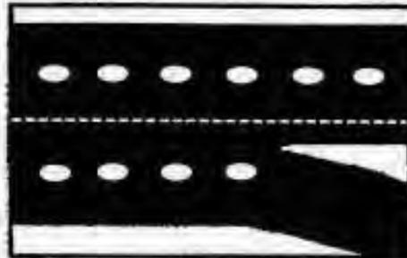
**SIPR** Separation in plane of coating on inner side of reinforcement. Can occur in either top or bottom sheet.
