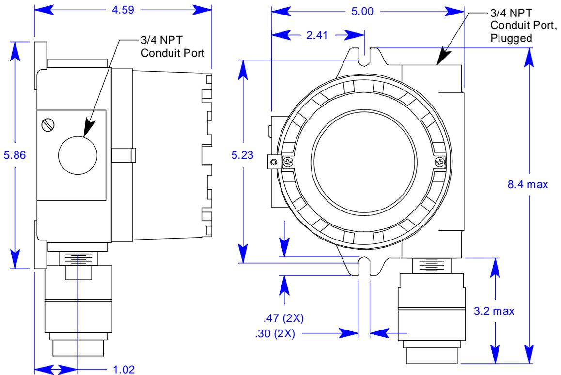
**Figure 15: Outline & Mounting Dimensions, CSA Type H<sub>2</sub>S, CO, and Oxygen**
