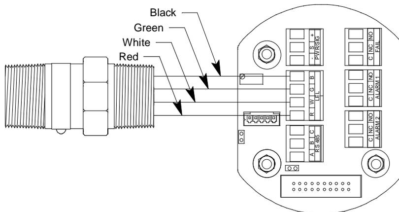
**Figure 18: Combustible IR/CO<sub>2</sub> Detector Wiring**
