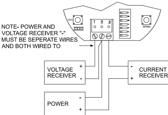
Figure 4: Simultaneous Current and Voltage Output Wiring
