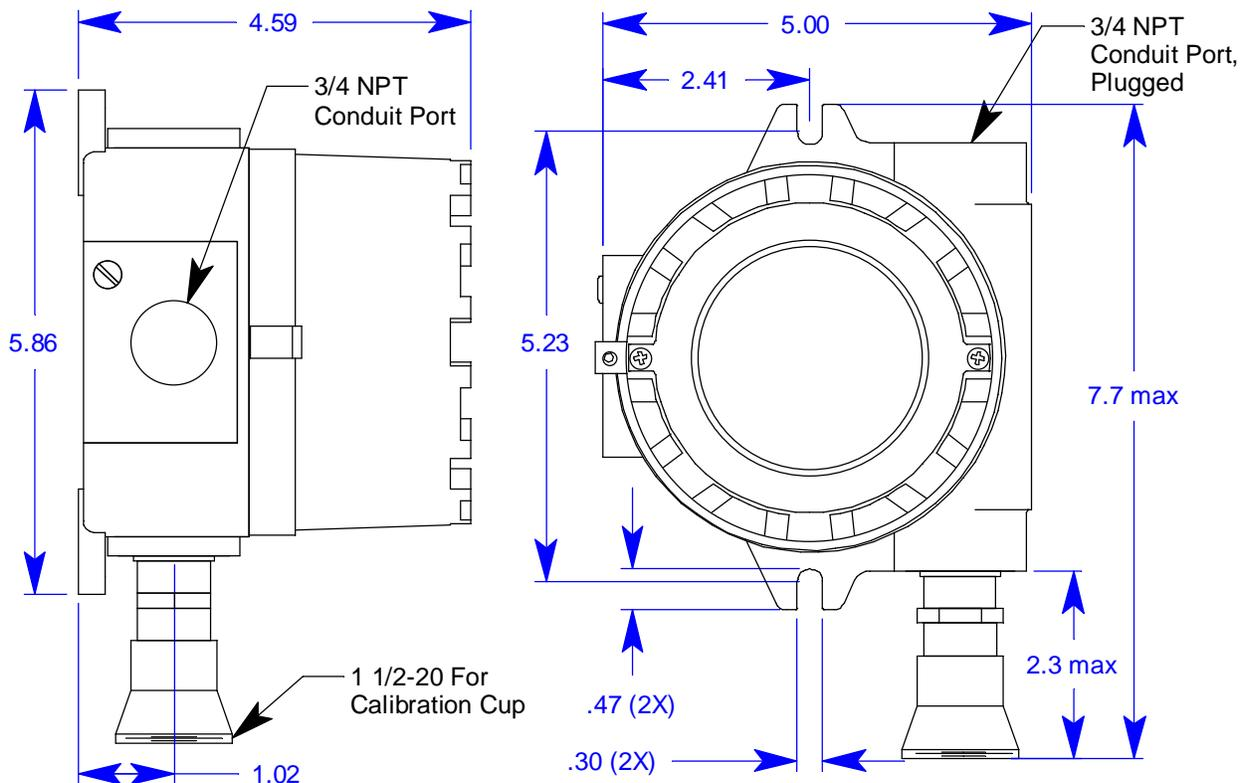
Figure 11: Outline & Mounting Dimensions, Catalytic LEL
