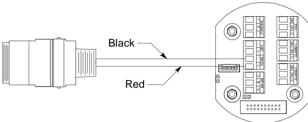
**Figure 23: H<sub>2</sub>S/CO Detector Wiring, CSA**
