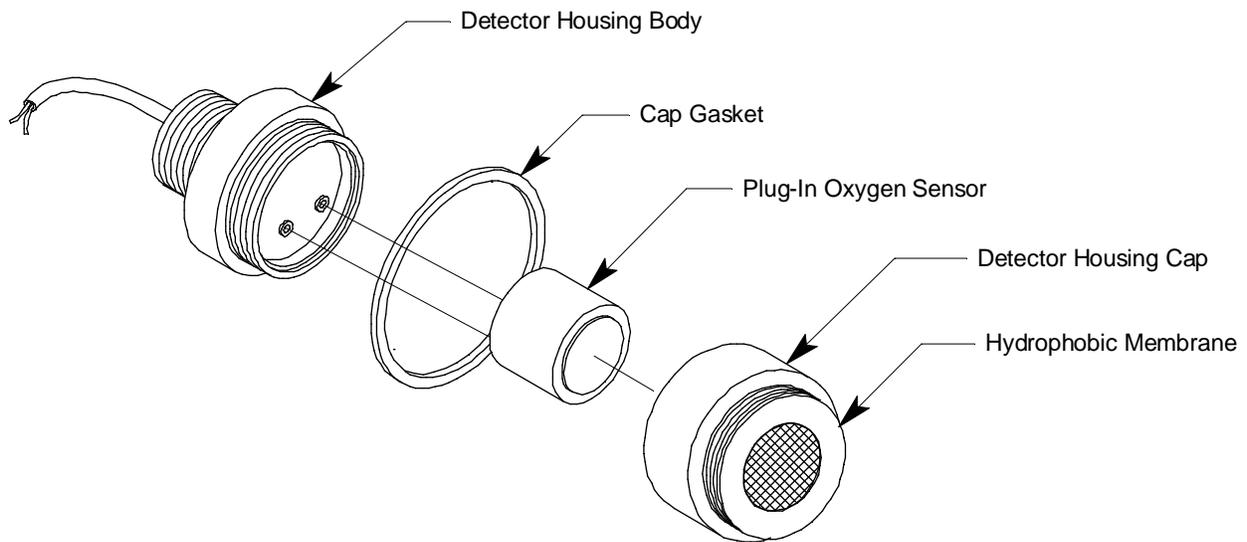
**Figure 3: 65-2494RK Oxygen Detector, Non-Explosion Proof, Capillary Type
