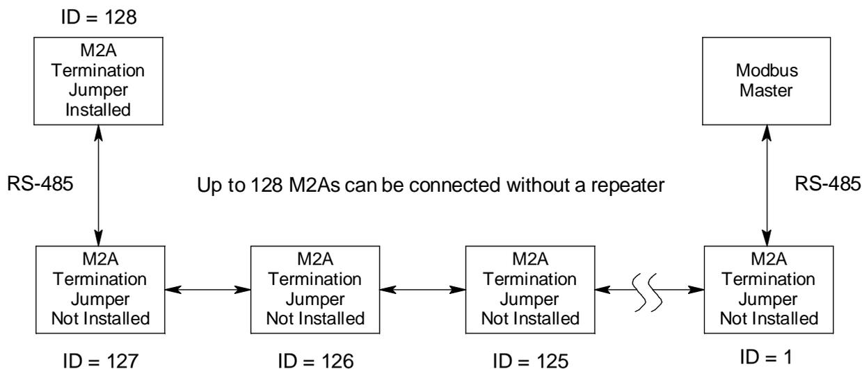
**Figure 29: Multiple M2As in a Daisy Chain Configuration**
