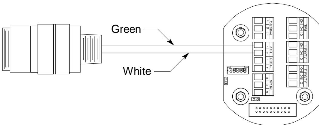
**Figure 21: CSA Capillary Type Oxygen Detector Wiring**
