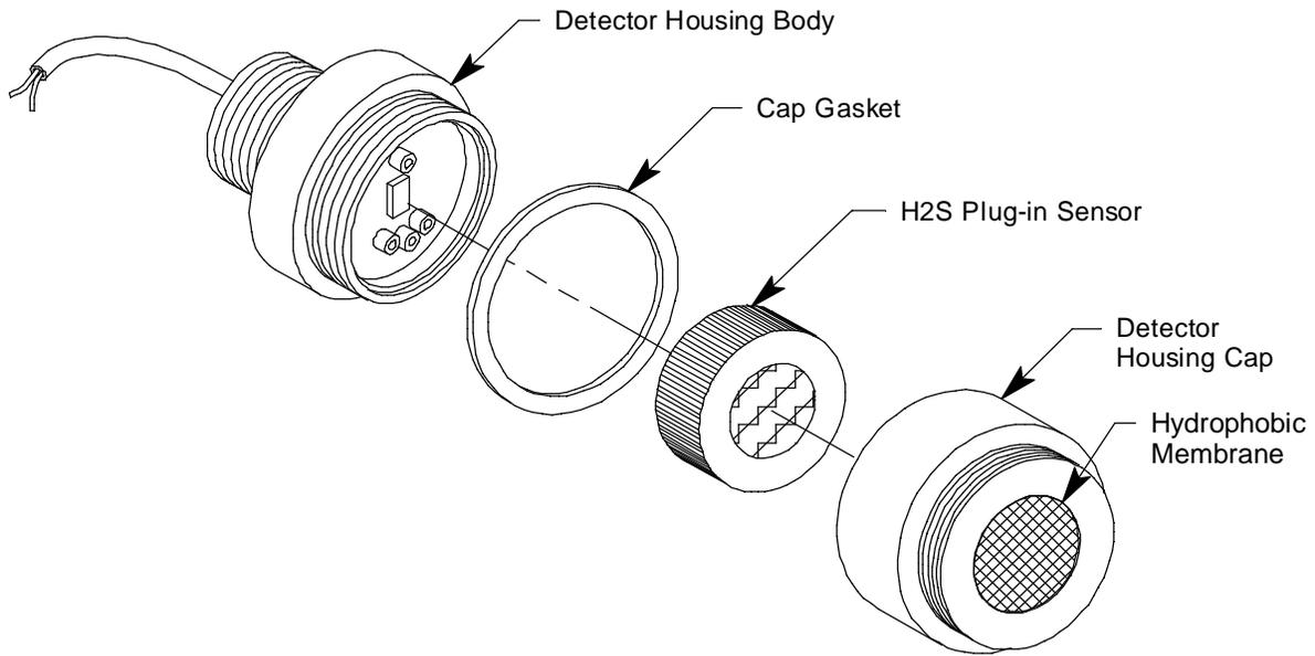
**Figure 7: 65-2495RK H<sub>2</sub>S Detector Non-Explosion Proof**
