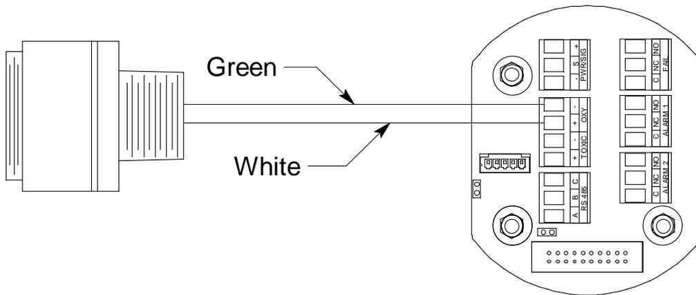
**Figure 22: Capillary Type Replaceable Sensor Oxygen Detector Wiring**
