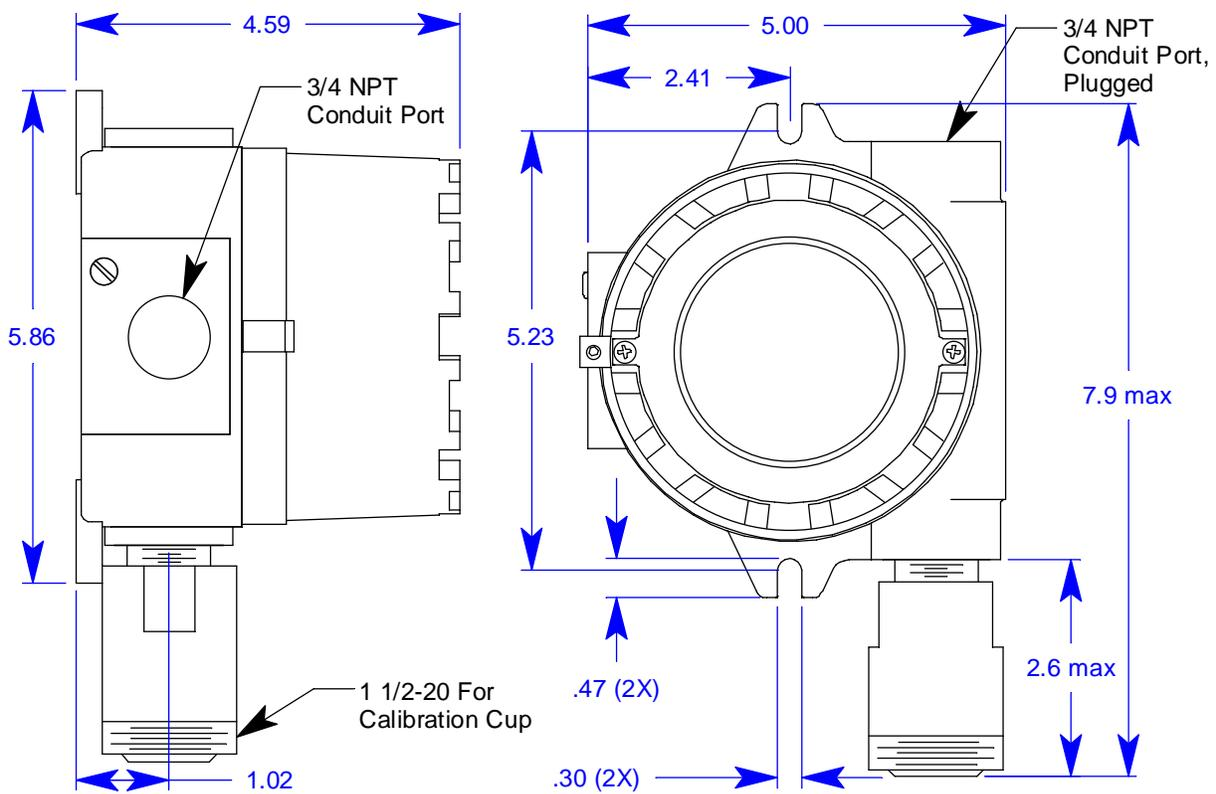
**Figure 13: Outline & Mounting Dimensions, Oxygen, Partial Pressure Type**
