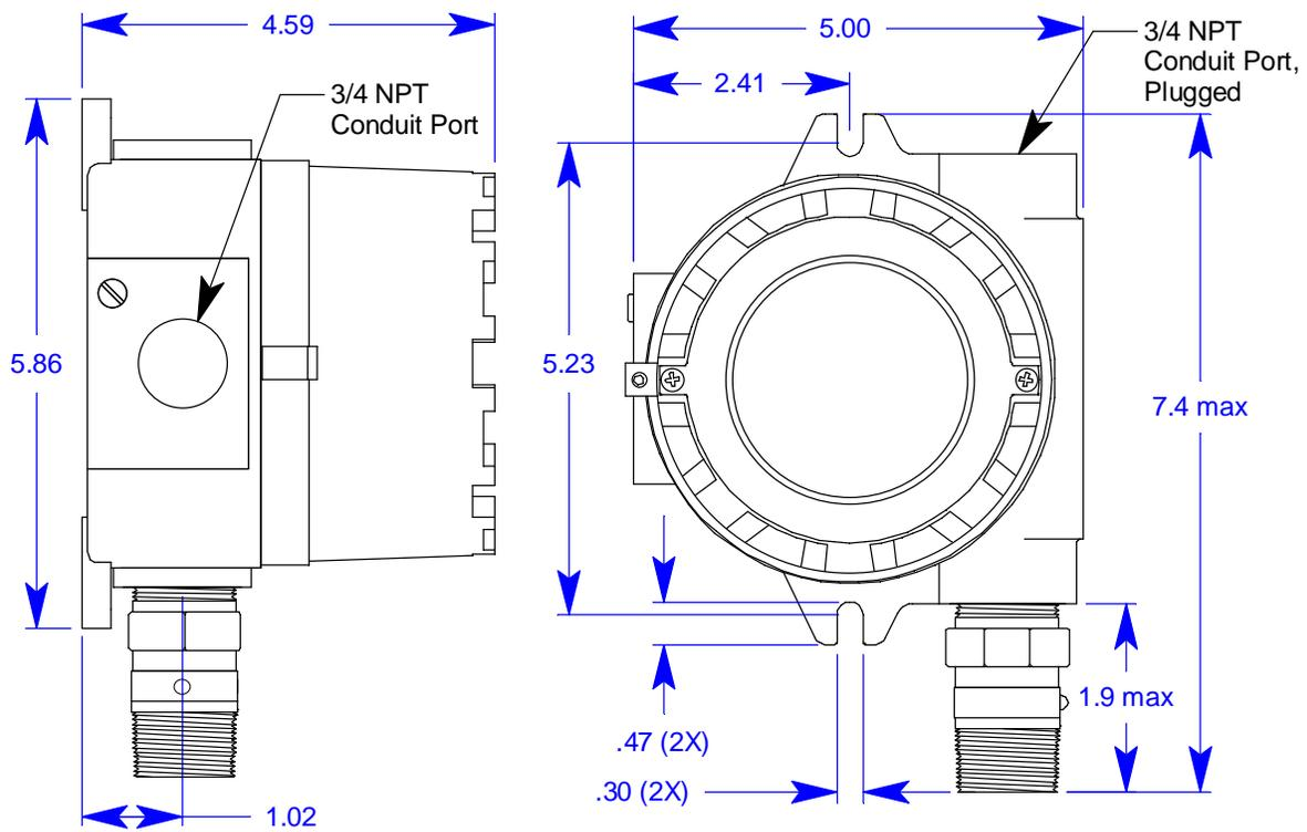
**Figure 12: Outline & Mounting Dimensions, IR Combustible & CO<sub>2</sub>**
