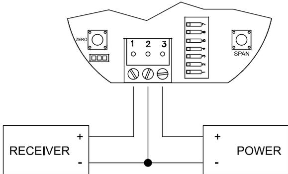
Figure 3: Voltage Output Wiring
