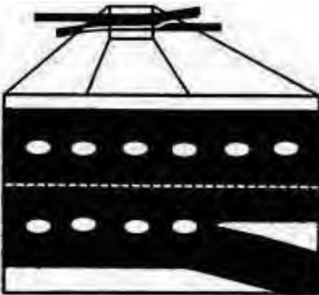
**SIPR** Separation in plane of reinforcement. Can occur in either top or bottom sheet.
