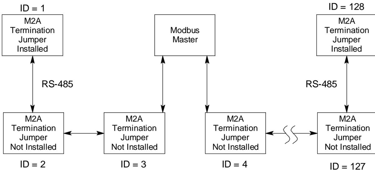
Up to 128 M2As can be connected without a repeater
