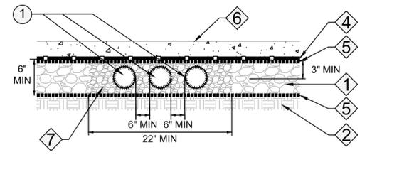
TYPICAL TRIPLE 2" PIPE SECTION
