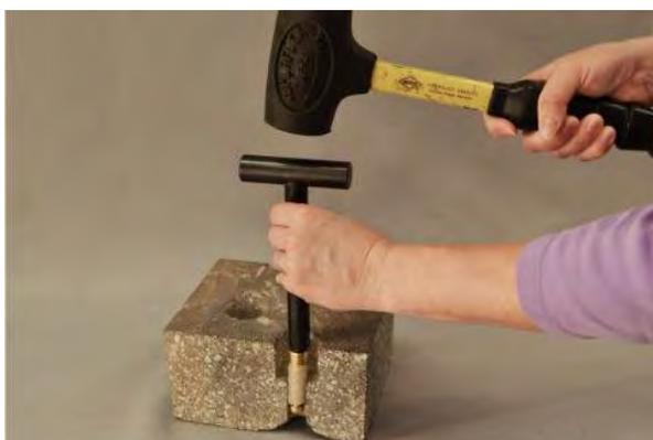
**Figure 3.** Flush-mount installation.
