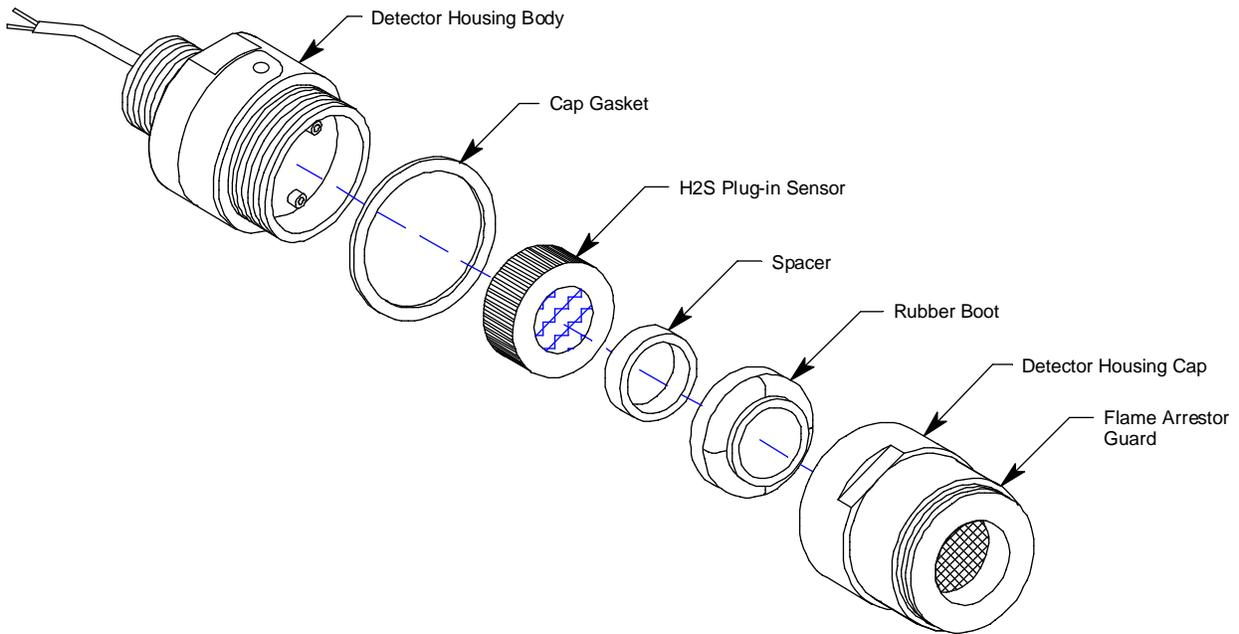
**Figure 6: 65-2428 H<sub>2</sub>S Detector, CSA**
