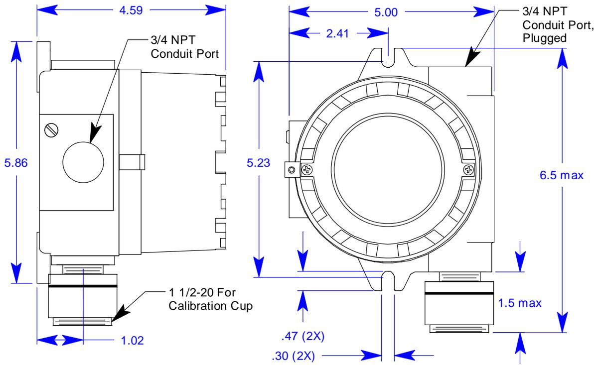
**Figure 14: Outline & Mounting Dimensions, Replaceable Sensor, Non Explosion Proof, H<sub>2</sub>S, CO, and Oxygen**
