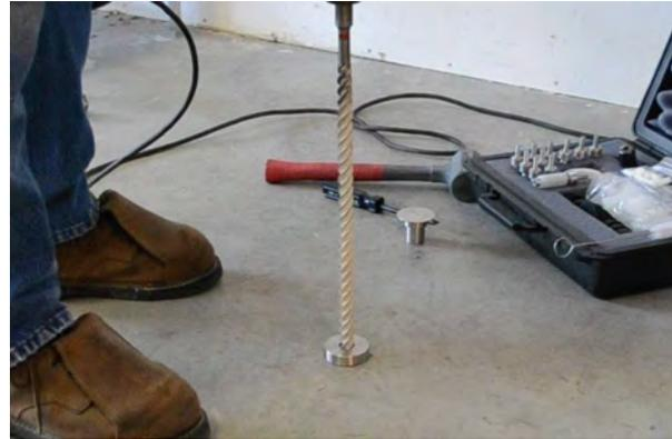
**Figure 4.** Using the Drilling Guide.
