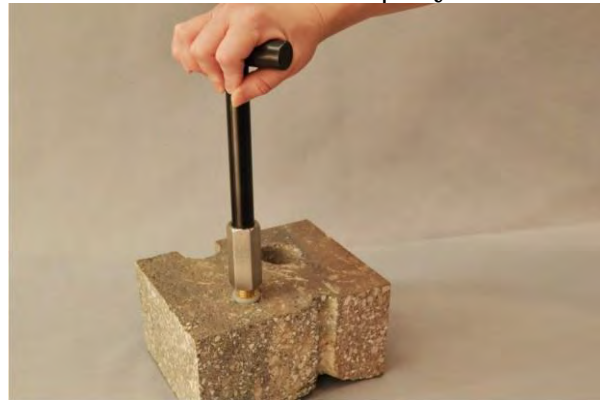
Figure 7. Removing the VAPOR PIN®
