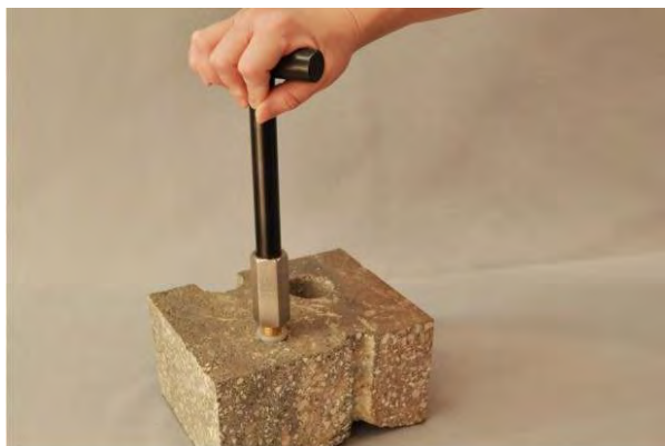
Figure 7. Removing the Vapor Pin™.
