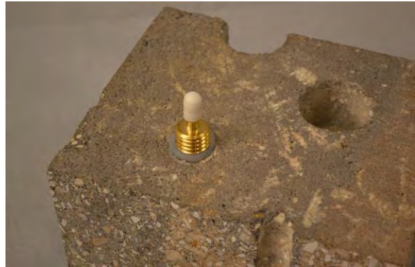
Figure 3. Installed VAPOR PIN®
