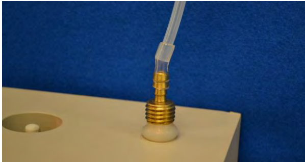
Figure 5. VAPOR PIN® sample connection
