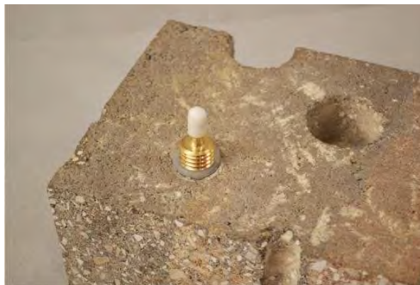
Figure 4. Installed Vapor Pin™.
