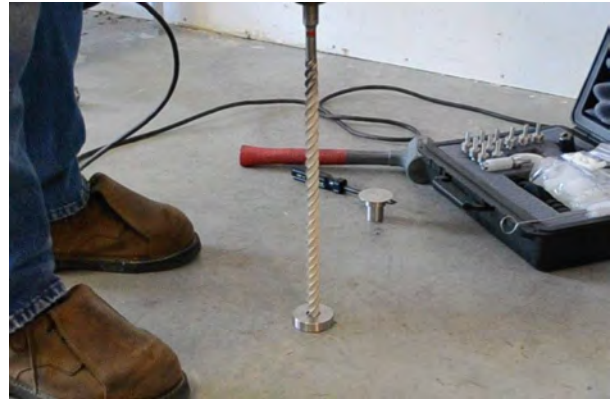
Figure 4. Using the Drilling Guide.
