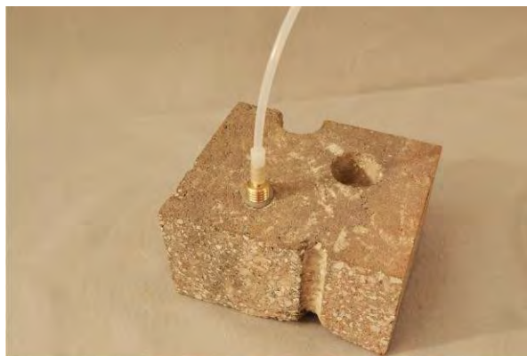
Figure 5. Vapor Pin™ sample connection.
