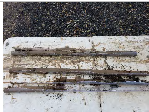
Photo 20. Soil cuttings from BH-08; 0 to 12 ft, 0 ft at bottom right, 12 ft at top left.
