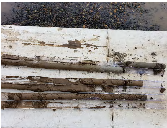
Photo 33. Soil cuttings from BH-14; 0 to 12 ft, 0 ft at bottom right, 12 ft at top left.
