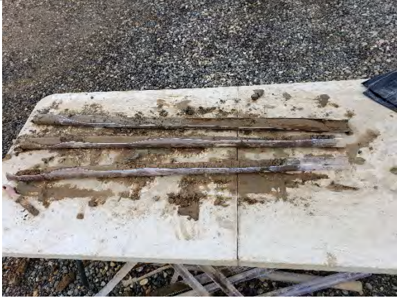
Photo 9. Soil cuttings from BH-04; 0 to 12 ft, 0 ft at bottom right, 12 ft at top left.
