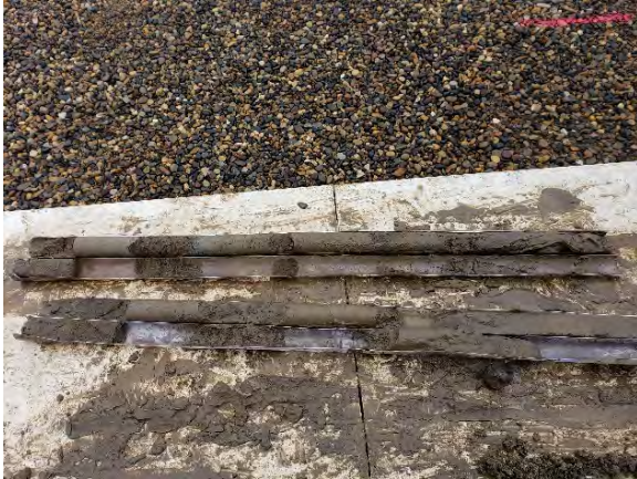
Photo 5. Soil cuttings from BH-02; 12 to 20 ft, 12 ft at bottom right, 20 ft at top left.
