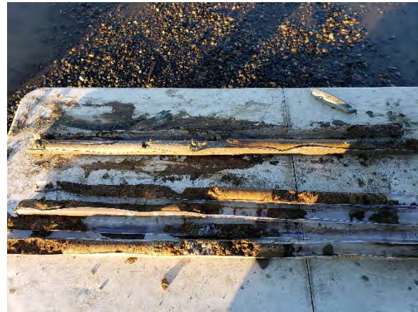
Photo 24. Soil cuttings from BH-10; 0 to 12 ft, 0 ft at bottom right, 12 ft at bottom left.
