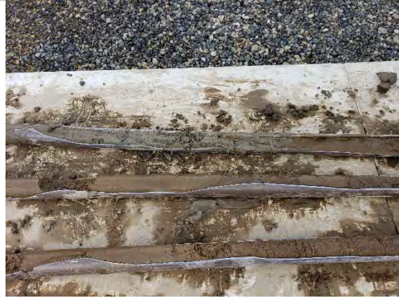
Photo 10. Closeup of soil cuttings from 8 to 12 ft, where soils turn grey.
