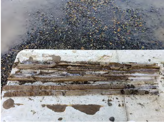
Photo 29. Soil cuttings from BH-12; 0 to 12 ft, 0 ft at bottom right, 12 ft at top left.
