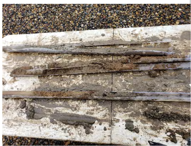
Photo 2. Soil cuttings from BH-01; 0 to 12 ft; 0 ft at bottom right, 12 ft at top left.
