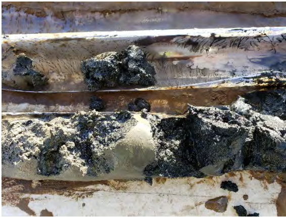
Photo 27. Closeup of soil cuttings from BH-11, where discoloration (black and grey) and odors first appeared.
