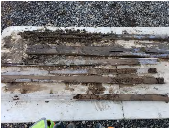
Photo 7. Soil cuttings from BH-03; 0 to 20 ft, 0 ft at bottom right, 20 ft at top left.
