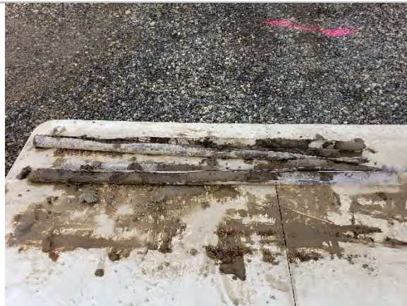
Photo 14. Soil cuttings from BH-05; 12 to 20 ft, 12 ft at bottom right, 20 ft at top left.
