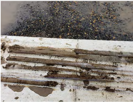
Photo 31. Soil cuttings from BH-13; 0 to 12 ft, 0 ft at bottom right, 12 ft at top left.
