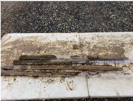
Photo 17. Soil cuttings from BH-06; 12 to 20 ft, 12 ft at bottom right, 12 ft at top left.
