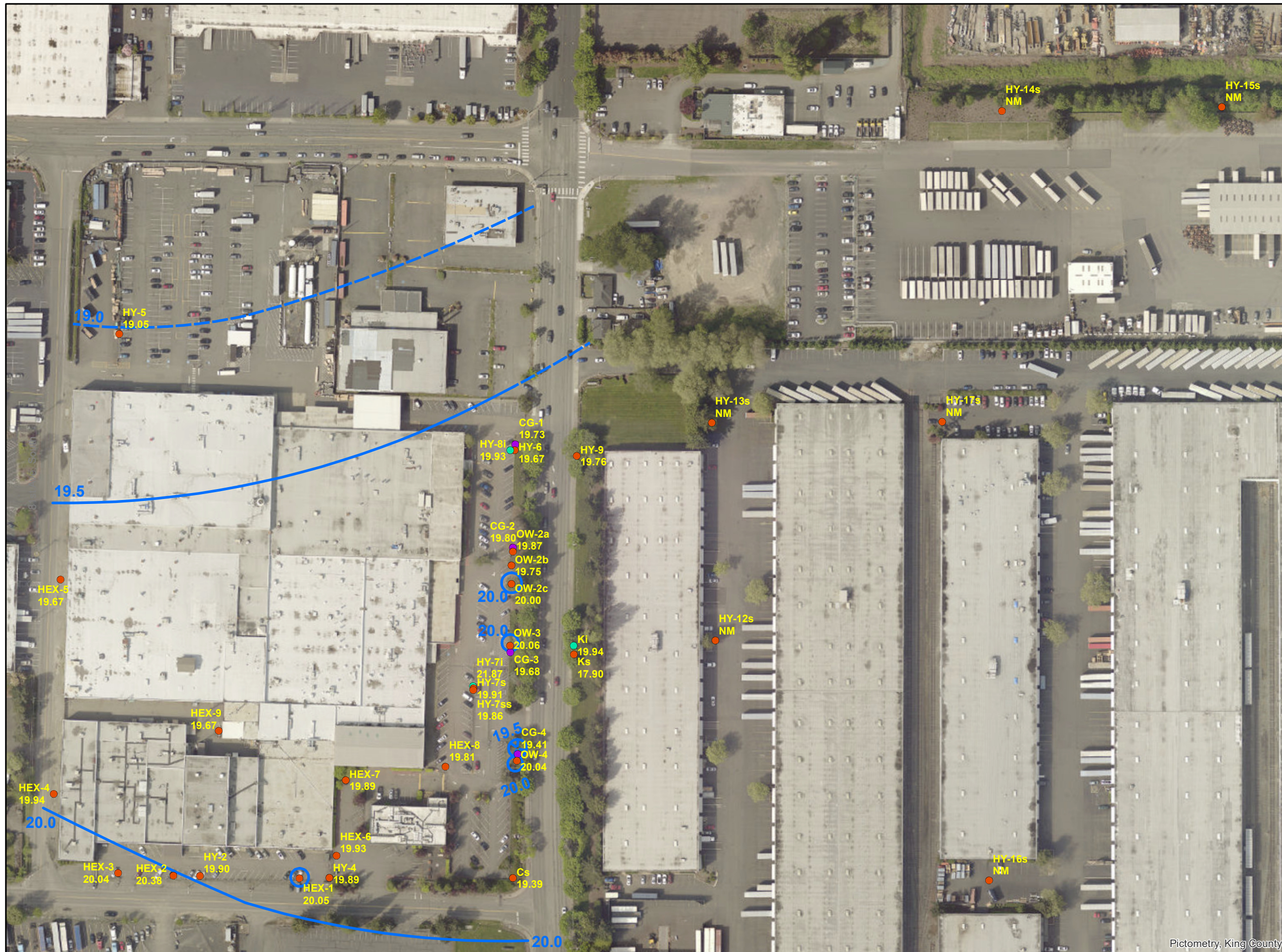
Figure 7 Contour Map of Shallow Groundwater Elevations (September 13-16, 2021) Plant 1 and Vicinity
