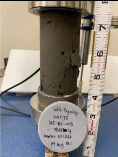
Picture Date: Thursday 10/07/2021 Picture Taken By: Matt Polsky Picture Location: Chelmsford, Massachusetts Project Name: USG Puyallup Pilot Study Project Description: ISS-A1-C13 UCS 14-day break
