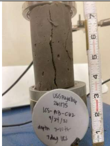
Picture Date: Friday 10/01/2021 Picture Taken By: Alan Smith Picture Location: Chelmsford, Massachusetts Project Name: USG Puyallup Pilot Study Project Description: ISS-A3-C62 UCS 7-day break
