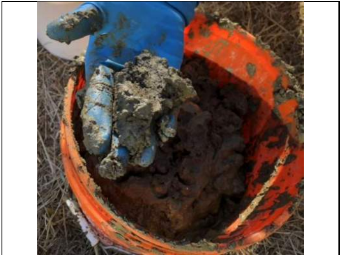
Picture Date: Thursday 09/23/2021 Picture Taken By: Matt Schultz Picture Location: Puyallup, Washington Project Name: USG Puyallup Site Project Description: ISS-2 Sample depth 20-23 ft bgs.
