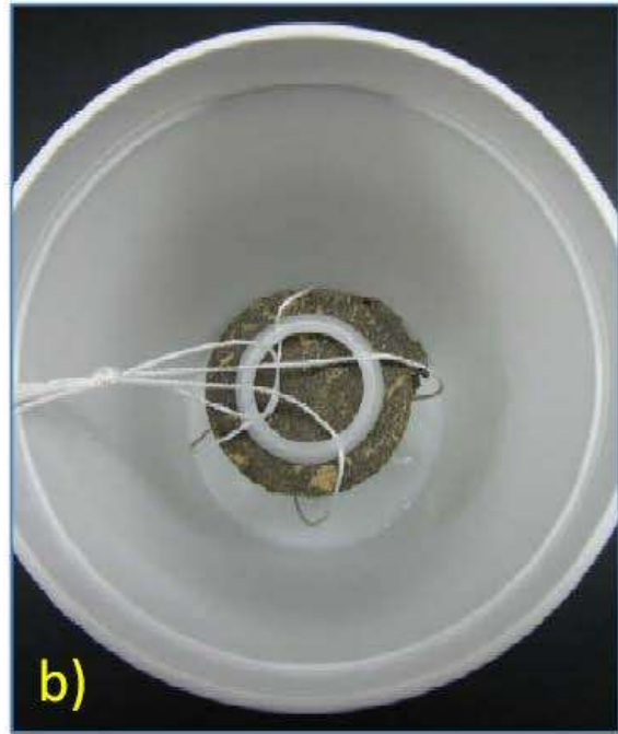
b) Sample Centered in Eluant (top view)
