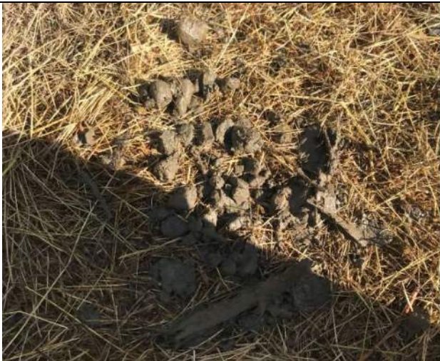
Picture Date: Friday 09/24/2021 Picture Taken By: Haley Provinsal Picture Location: Puyallup, Washington Project Name: USG Puyallup ISS Pilot Study Project Description: ISS-3 Sample depth 13-17 ft bgs 3/8" Sieve retained material (gravel, wood, roots)
