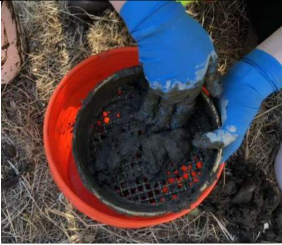
Picture Date: Thursday 09/23/2021 Picture Taken By: Matt Schultz Picture Location: Puyallup, Washington Project Name: USG Puyallup Site Project Description: Sieving ISS-2 Sample depth 10-13 ft bgs.
