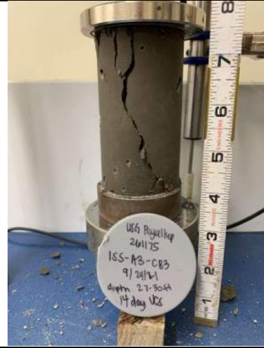
Picture Date: Friday 10/08/2021 Picture Taken By: Matt Polsky Picture Location: Chelmsford, Massachusetts Project Name: USG Puyallup Pilot Study Project Description: ISS-A2-C83 UCS 14-day break
