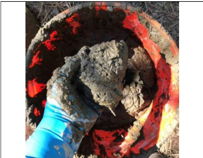
Picture Date: Friday 09/24/2021 Picture Taken By: Haley Provinsal Picture Location: Puyallup, Washington Project Name: USG Puyallup ISS Pilot Study Project Description: ISS-5 Sample depth 7-10 ft bgs.
