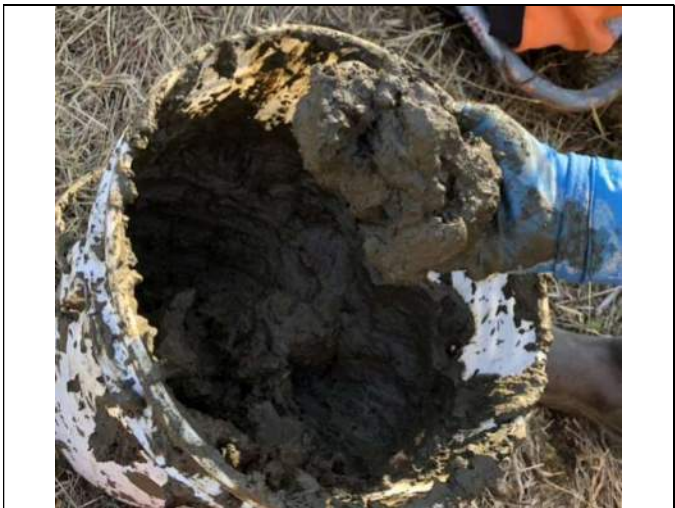
Picture Date: Thursday 09/23/2021 Picture Taken By: Matt Schultz Picture Location: Puyallup, Washington Project Name: USG Puyallup ISS Pilot Study Project Description: ISS-2 Sample depth 10-13 ft bgs.
