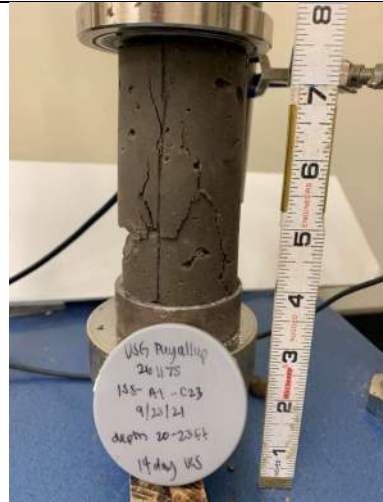
Picture Date: Thursday 10/07/2021 Picture Taken By: Matt Polsky Picture Location: Chelmsford, Massachusetts Project Name: USG Puyallup Pilot Study Project Description: ISS-A1-C23 UCS 14-day break
