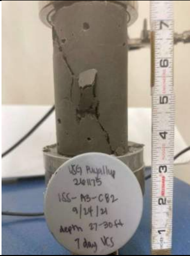
Picture Date: Friday 10/01/2021 Picture Taken By: Alan Smith Picture Location: Chelmsford, Massachusetts Project Name: USG Puyallup Pilot Study Project Description: ISS-A3-C82 UCS 7-day break
