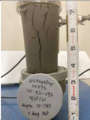
Picture Date: Friday 10/01/2021 Picture Taken By: Alan Smith Picture Location: Chelmsford, Massachusetts Project Name: USG Puyallup Pilot Study Project Description: ISS-A2-C42 UCS 7-day break
