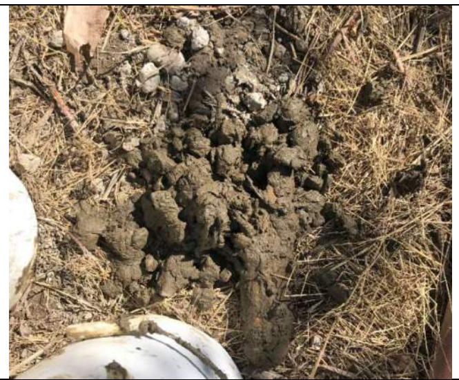
Picture Date: Friday 09/24/2021 Picture Taken By: Haley Provinsal Picture Location: Puyallup, Washington Project Name: USG Puyallup ISS Pilot Study Project Description: ISS-5 Sample depth 27-30 ft bgs 3/8" Sieve retained material (gravel, cobbles, wood, twigs)
