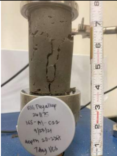
Picture Date: Thursday 09/30/2021 Picture Taken By: Alan Smith Picture Location: Chelmsford, Massachusetts Project Name: USG Puyallup Pilot Study Project Description: ISS-A1-C22 UCS 7-day break
