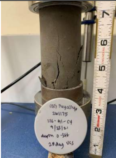
Picture Date: Thursday 10/21/2021 Picture Taken By: Matt Polsky Picture Location: Chelmsford, Massachusetts Project Name: USG Puyallup Pilot Study Project Description: ISS-A1-C4 UCS 28-day break
