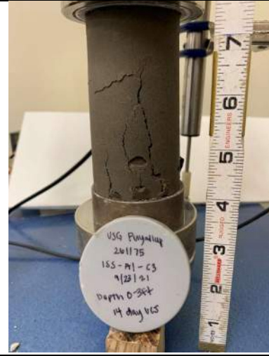
Picture Date: Thursday 10/07/2021 Picture Taken By: Matt Polsky Picture Location: Chelmsford, Massachusetts Project Name: USG Puyallup Pilot Study Project Description: ISS-A1-C3 UCS 14-day break
