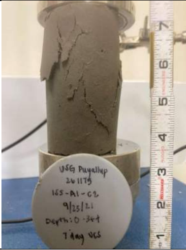
Picture Date: Thursday 09/30/2021 Picture Taken By: Alan Smith Picture Location: Chelmsford, Massachusetts Project Name: USG Puyallup Pilot Study Project Description: ISS-A1-C2 UCS 7-day break
