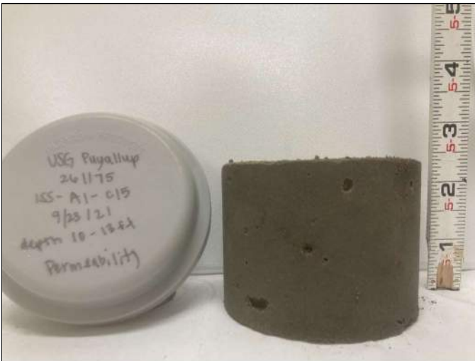
Picture Date: Thursday 11/18/2021 Picture Taken By: Matt Polsky Picture Location: Chelmsford, Massachusetts Project Name: USG Puyallup Pilot Study Project Description: ISS-A1-C15 Permeability Test
