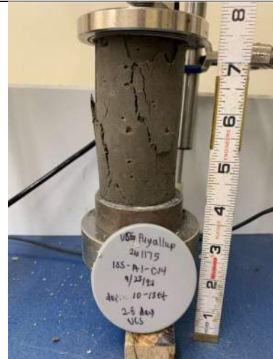
Picture Date: Thursday 10/21/2021 Picture Taken By: Matt Polsky Picture Location: Chelmsford, Massachusetts Project Name: USG Puyallup Pilot Study Project Description: ISS-A1-C14 UCS 28-day break
