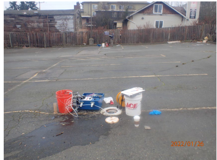
Low-flow purge and sampling set up on Well #7 (foreground) and Well #5 (background).
