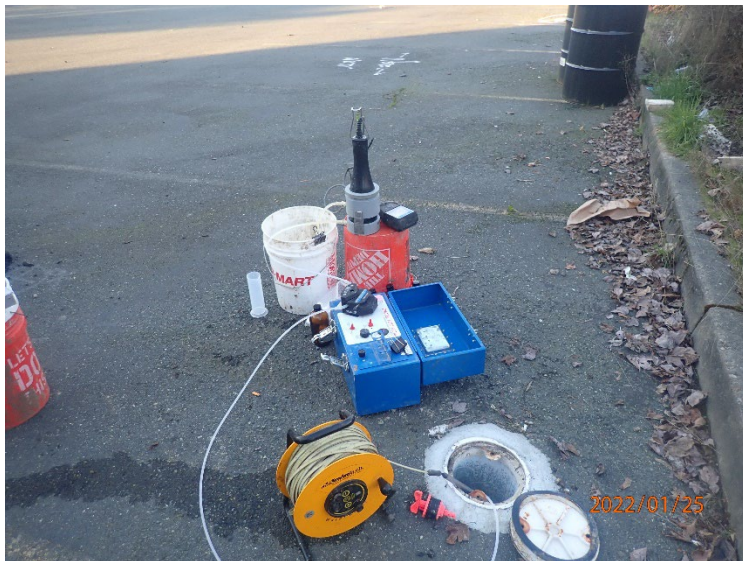
Low-flow purge and sampling set up on Well #10 next to eastern site boundary using a peristaltic pump (blue box).
