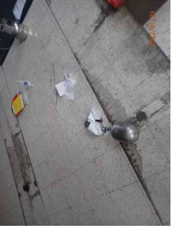
Sampling SUB01 using a certified 3-L SUMMA canister. Isopropyl alcohol (IPA) -saturated rags placed over fittings and vapor pin for leak checking.
