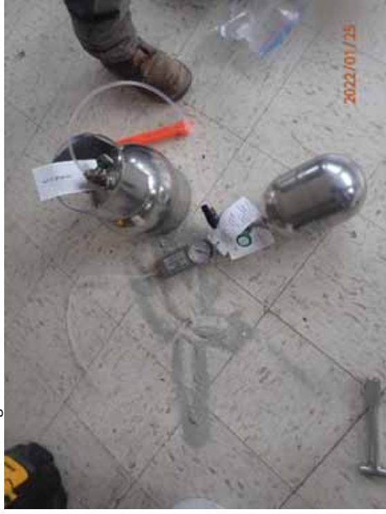
Sampling SUB01 using a certified 3-L SUMMA canister. Isopropyl alcohol (IPA) -saturated rags placed over fittings and vapor pin for leak checking.
