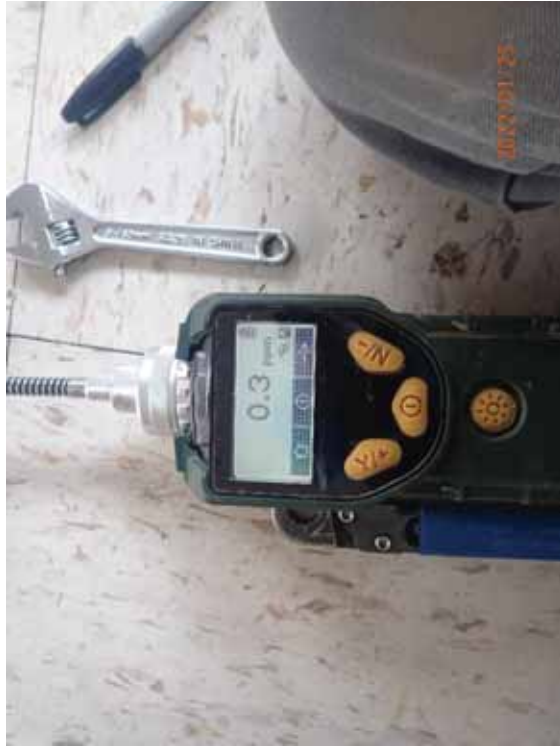
Measuring sub-slab VOCs using a PID following sample collection.
