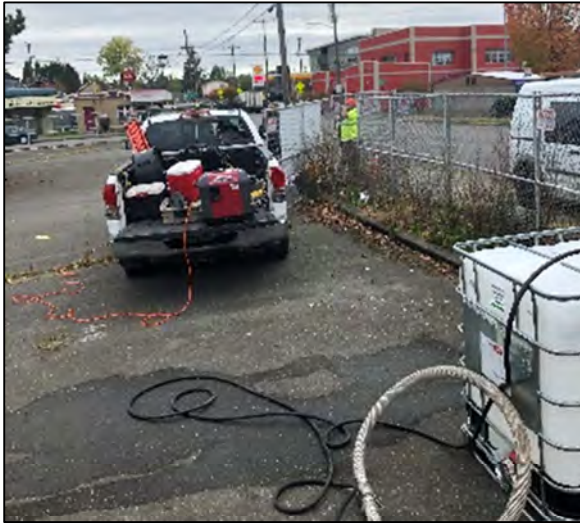
Photo 1: Water source storage tote and well extraction setup.
