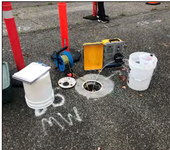
Photo 4: ROI data collection setup on downgradient wells.
