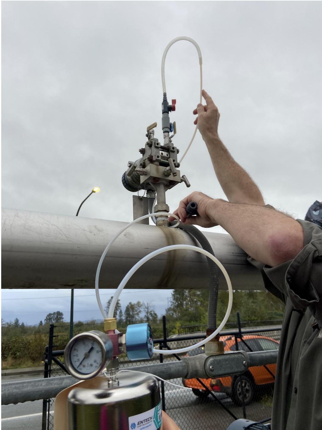
Figure 2. Sampling at South Blower. Initial vacuum at 30 inches of mercury.
