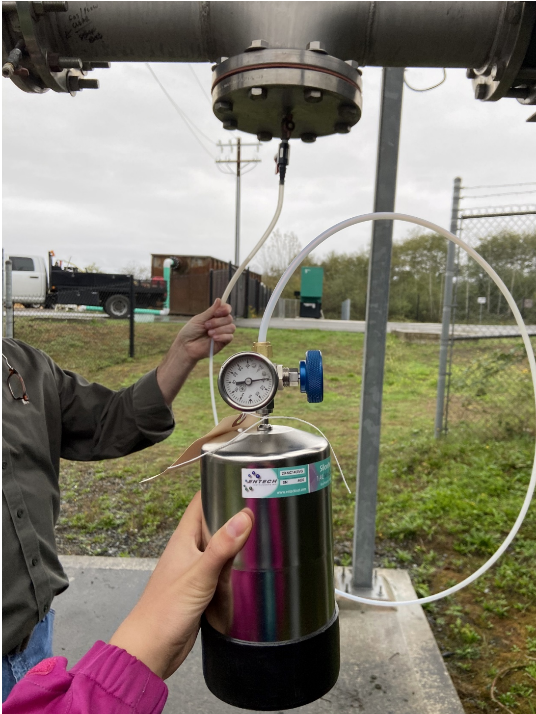
Figure 4. Sampling at North Blower. Initial vacuum at 30 inches of mercury.
