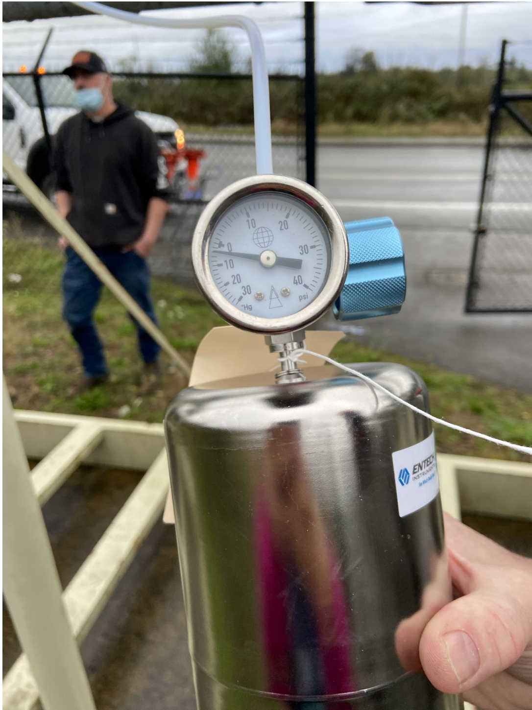
Figure 3. Pressure gauge after sample was grabbed at South Blower. Final vacuum at 4 inches of mercury.
