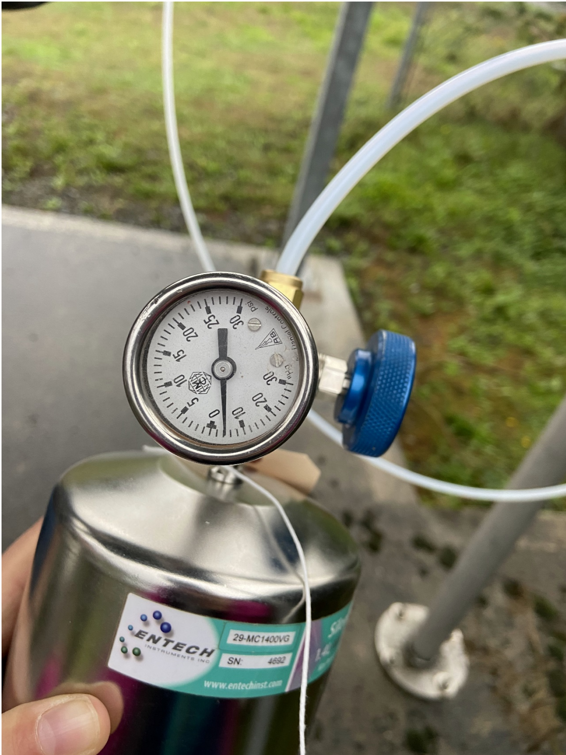
Figure 5. Pressure gauge after sample was grabbed at North Blower. Final vacuum at 4 inches of mercury.
