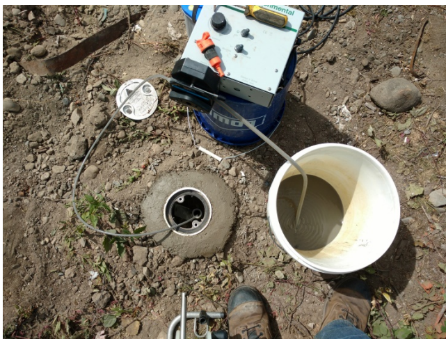
Purging of MW5A
