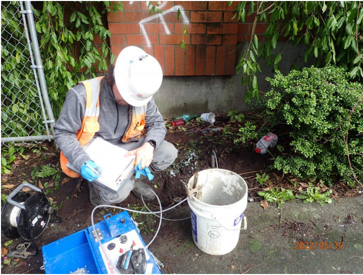
Reconnaissance ground water sample collected from EB01 with a peristaltic pump using low-flow purge and sampling methodology.
