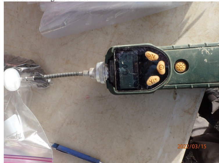
A PID being used to measure headspace for field screening of soil contaminants.
