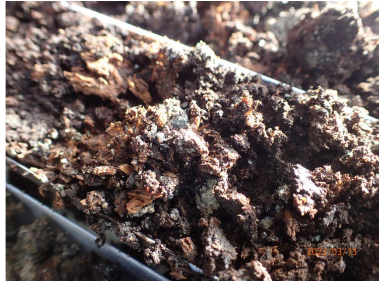
Close-up view of thick layer of peat encountered in all borings.
