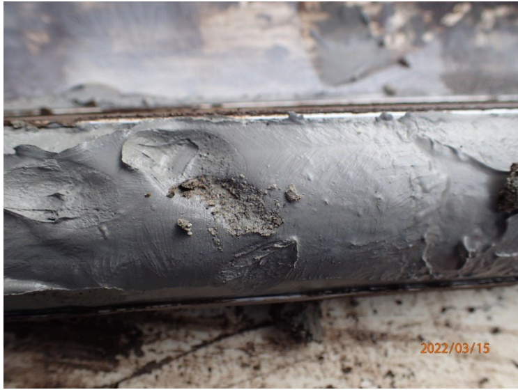
Gray, highly plastic clay soils were encountered at the bottom of the borings.
