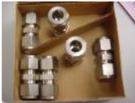
Figure 4. Swagelok ® connectors (image from equipsales.com)
