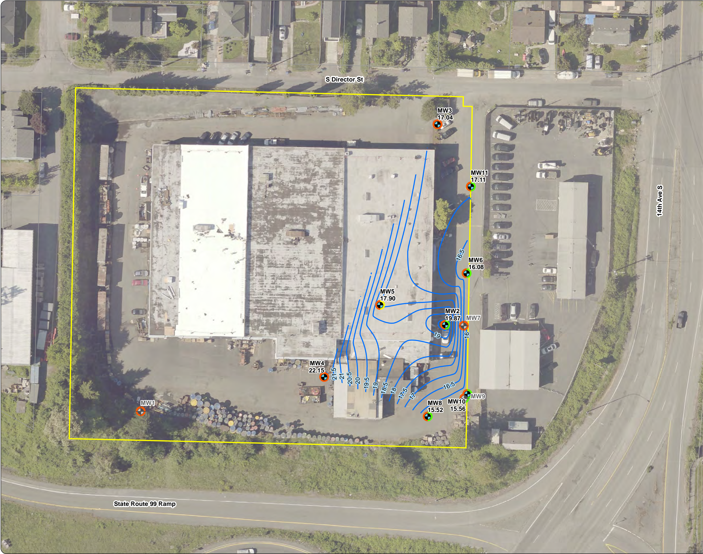
Figure C-3 Potentiometric Surface Map Shallow Water Bearing Zone December 2019 Precision Engineering, Inc. Seattle, Washington DRAFT
