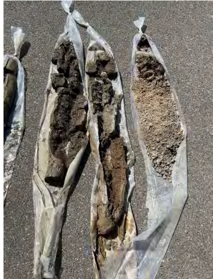
Photo 4. MW-6D soil cores, from about 2.5 ft below ground surface (right) to about 15 ft below ground surface (left).
