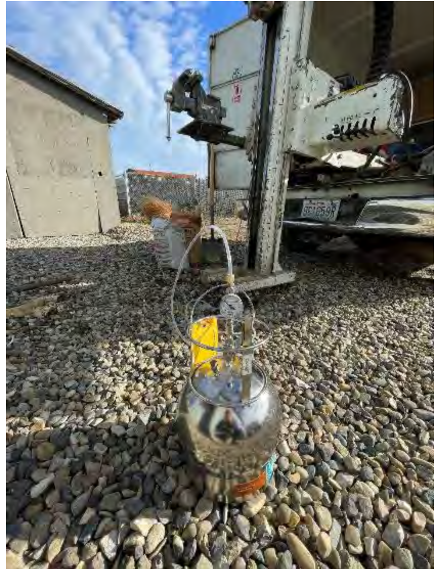
Photo 16. Collecting soil vapor intrusion sample VI2.5-02 (sample collected at 4-ft below ground surface).
