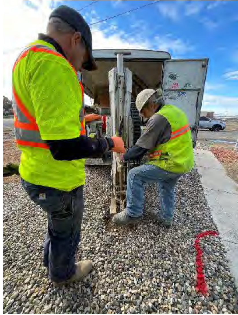
Photo 14. Soil vapor intrusion investigation location VI2.5-01 (sample collected at 4-ft below ground surface).
