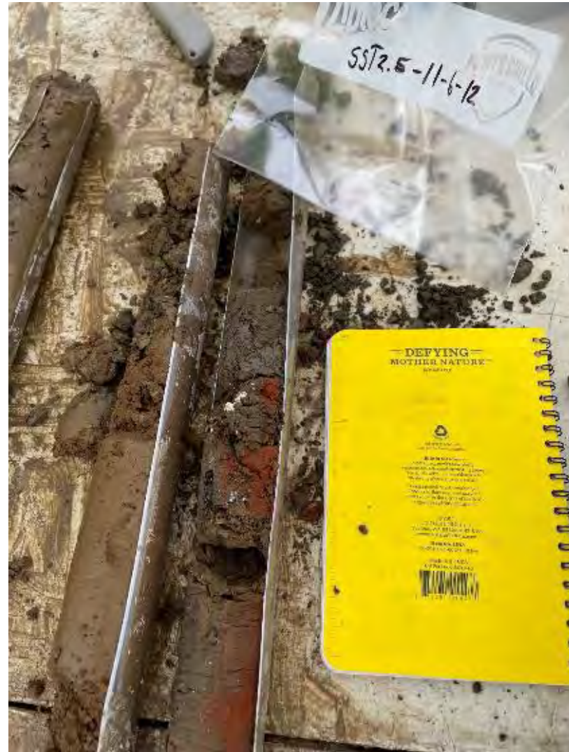
Photo 10. Soil suitability testing grab sample collected with GeoProbe (SST2.5-11-6-12).
