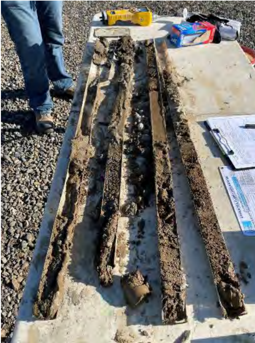
Photo 11. Onsite soil vapor headspace screening investigation conducted with GeoProbe. Borings from location SVH2.5-01, 0 feet (right) to 8 feet (left).
