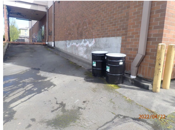
Well purge water was placed in DOT-approved drums pending disposal.
