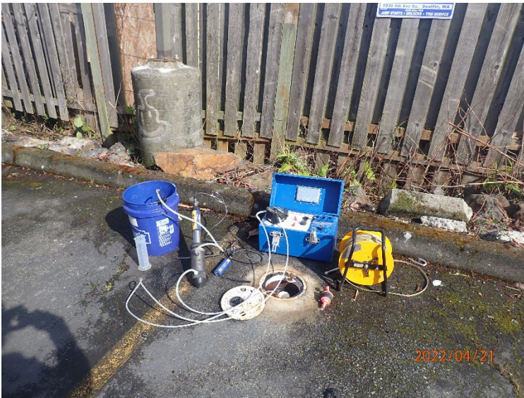
Low-flow purge and sampling set up on Well #12 next to northern site boundary using a peristaltic pump (blue box).
