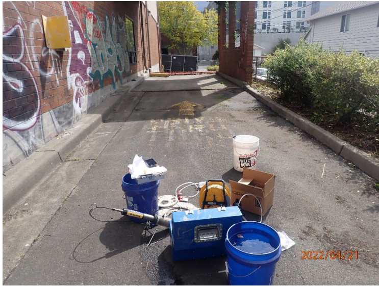
Low-flow purge and sampling of Well #3 – looking south.
