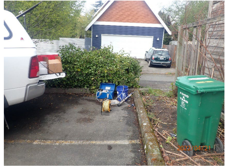
Low-flow purge and sampling set up on Well #6.
