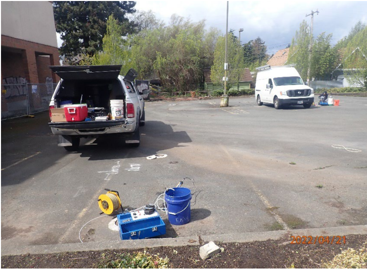
Gauging Well #10 with a depth to water meter, view looking west.
