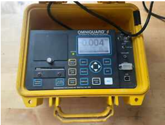
Photograph 3. An OmniGuard 4 micromanometer used to monitor differential pressure across the building foundation and VIMS barrier.
