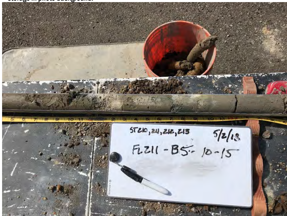
Photograph 13 – FL-211 – Boring location FL211-B5 showing soil core from 10 to 15 feet below ground surface. The concentration of cPAHs at 11.5-12 feet was > MTCA.
