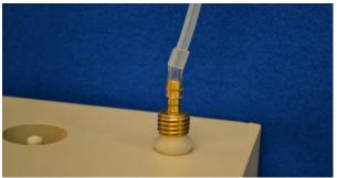
Figure 5. VAPOR PIN® sample connection
