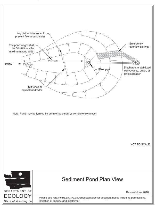
Figure 7.30: Sediment Pond Plan View
