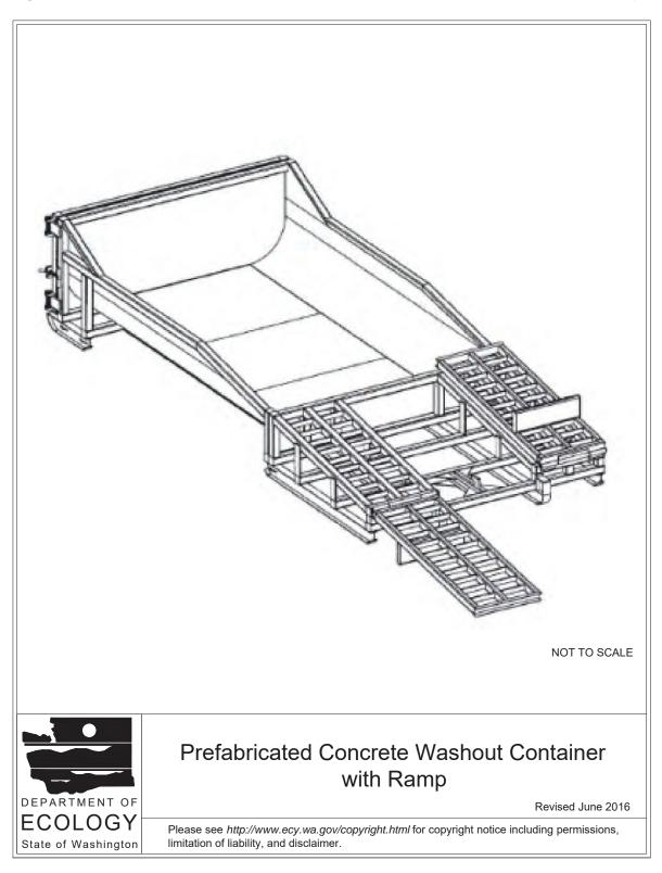
Figure 7.11: Prefabricated Concrete Washout Container with Ramp
