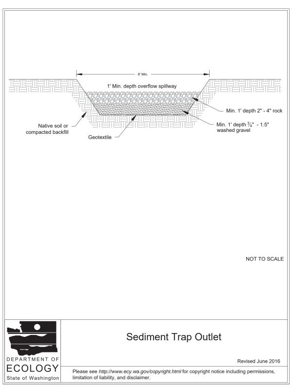
Figure 7.29: Sediment Trap Outlet
