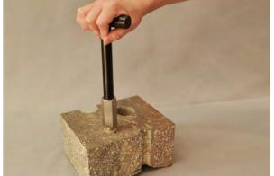
Figure 7. Removing the VAPOR PIN®
