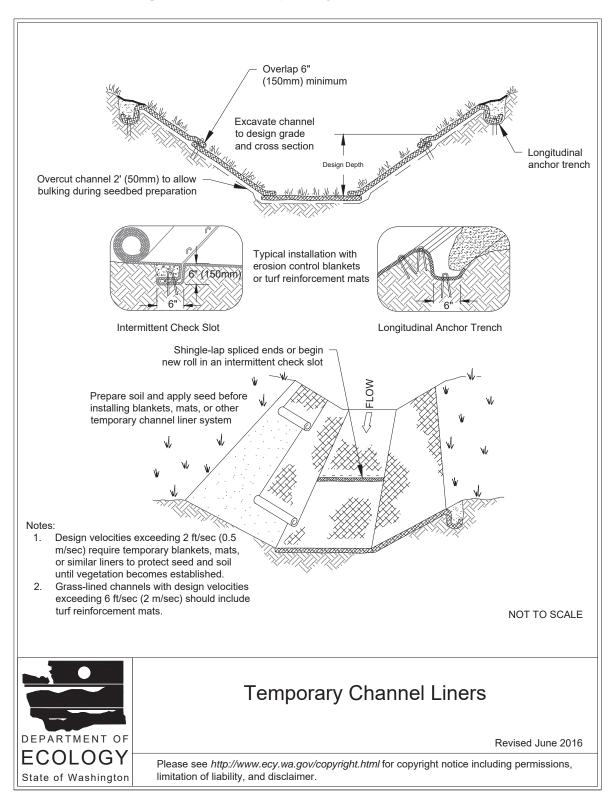
Figure 7.13: Temporary Channel Liners
