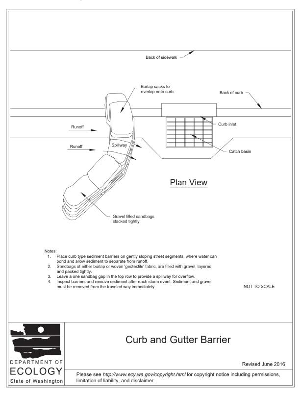
Figure 7.21: Curb and Gutter Barrier
