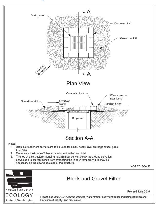
Figure 7.19: Block and Gravel Filter
