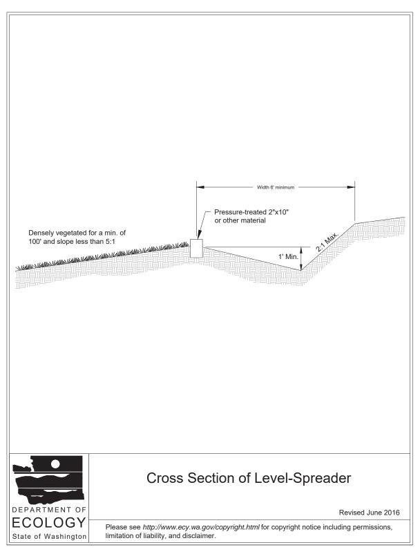
Figure 7.16: Cross Section of Level-Spreader
