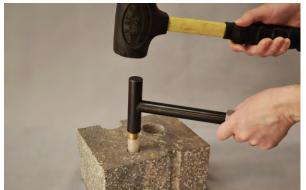
Figure 2. Installing the VAPOR PIN®
