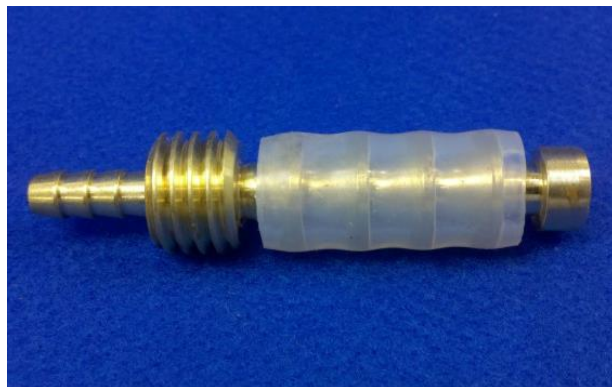
Figure 1. Assembled VAPOR PIN® sampling device
