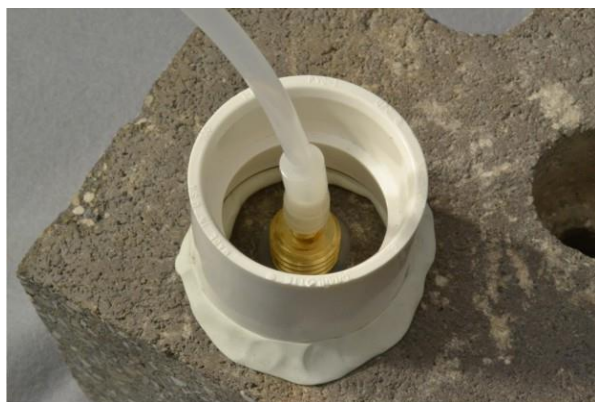
Figure 7. Removing the VAPOR PIN® sampling device
