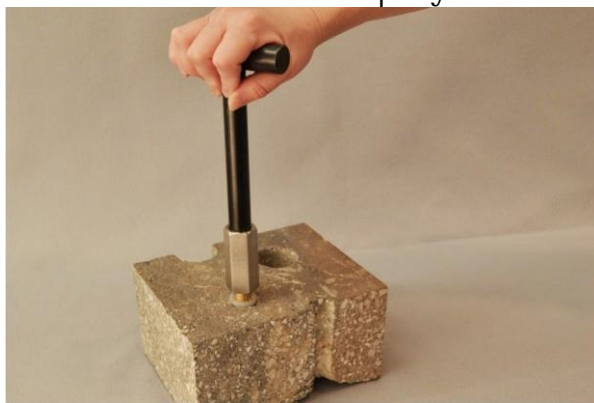
Figure 7. Removing the VAPOR PIN® sampling device
