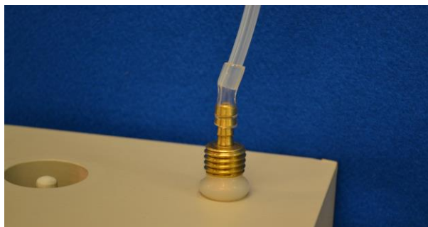
Figure 5. VAPOR PIN® sampling device sample connection
