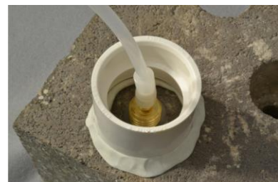
Figure 1. Water dam used for leak detection
