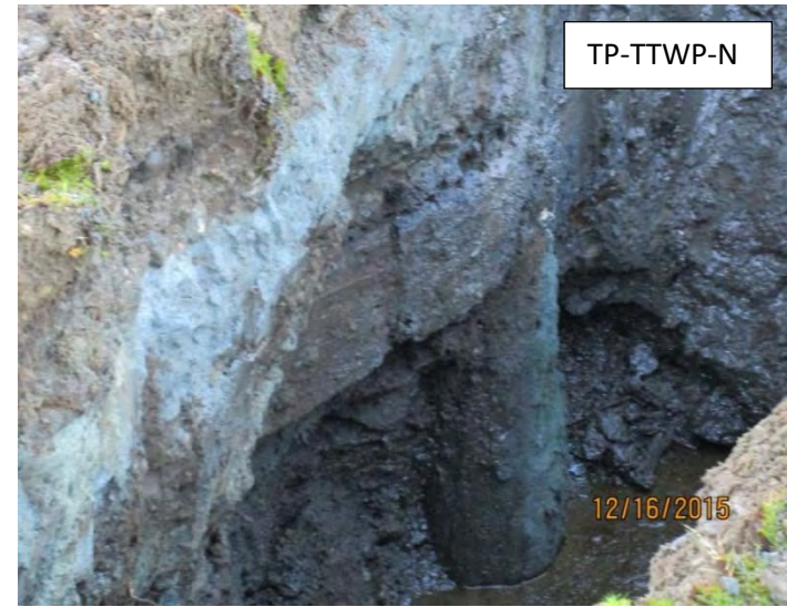
Woody debris in TP-TTWP-S (left) high volume of wooden piles and timbers. TP-TTWP-N (right) significant large dimensional lumber debris present.
