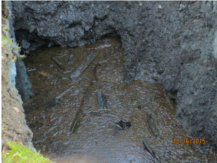
Photo 13: TP-TTWP-N - High volume of large dimensional woody debris in oil-stained saturated layer
