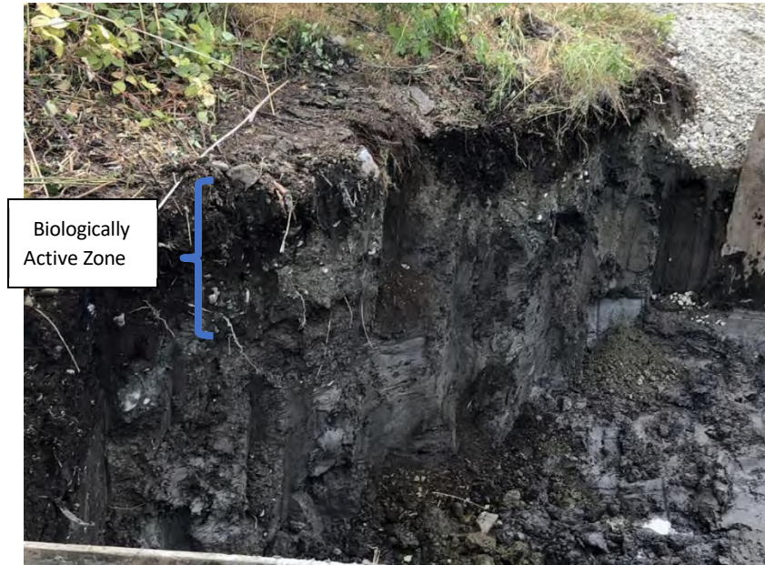
Figure 9: Cross Section of Sediments Showing Biologically Active Zone to Two Feet
