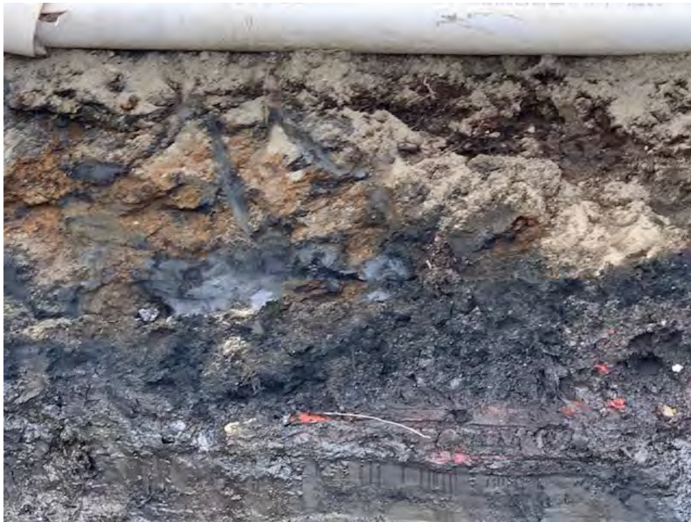
Figure 24: RAU B5: Close up Eastern sidewall at 0-5 feet – NOTE: Presence of “Shot” in center of photograph
