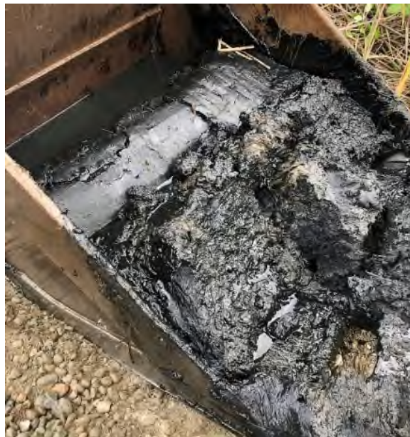
Figure 7: TPH-Impacted Soil Found in Ditch Sediment
