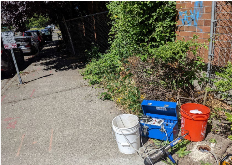
Purging and sampling EMW01 with a peristaltic pump and field meter with flow-through cell, view looking west.
