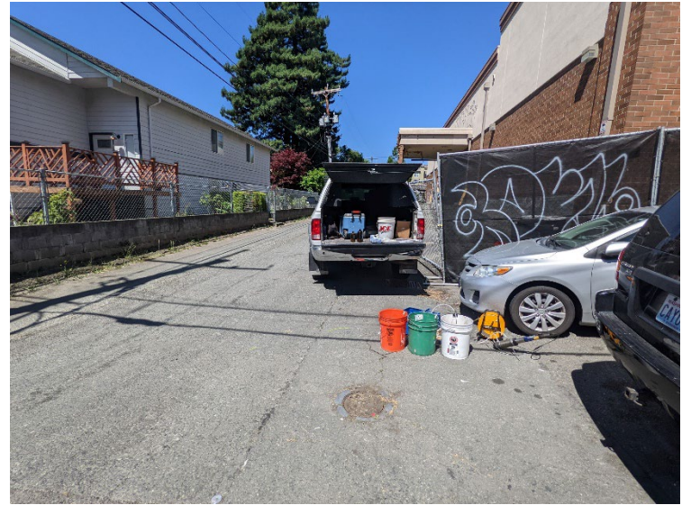
Low-flow purge and sampling set up on Well #2 in the southwestern corner of the site.
