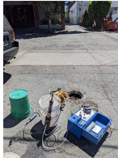
Low-flow purge and sampling at MW-8, view south.
