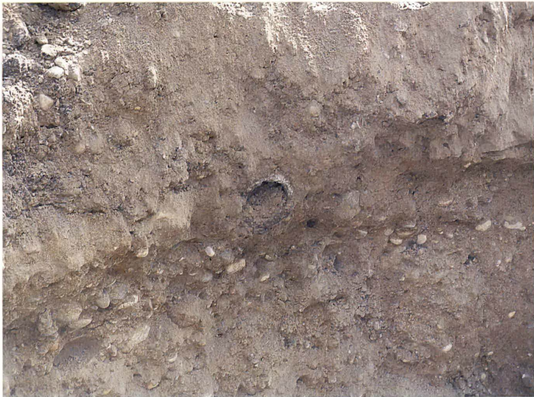
Photo 4. View of the shallow exposed surface near the center of the excavation (approximately 30 inches deep) showing one of the former utility lines present beneath the building extension. Note the horizon of stained soil immediately adjacent to this utility line.
