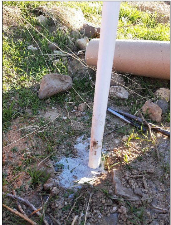
Photo 4: Bentonite seal used during sampling at location A-3. December 8, 2021
