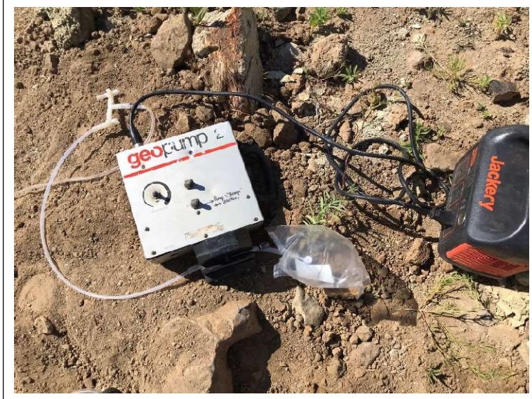
Filling a tedlar bag with the peristaltic pump.
