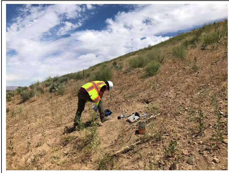
Measuring LFG with the Landtec GEM 5000 at location VP-2
