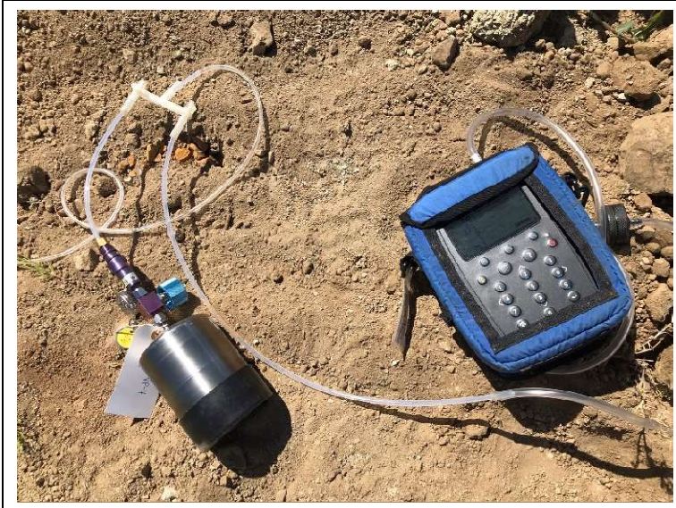
Example set up using a manifold connected to the GEM and summa canister at location VP-4
