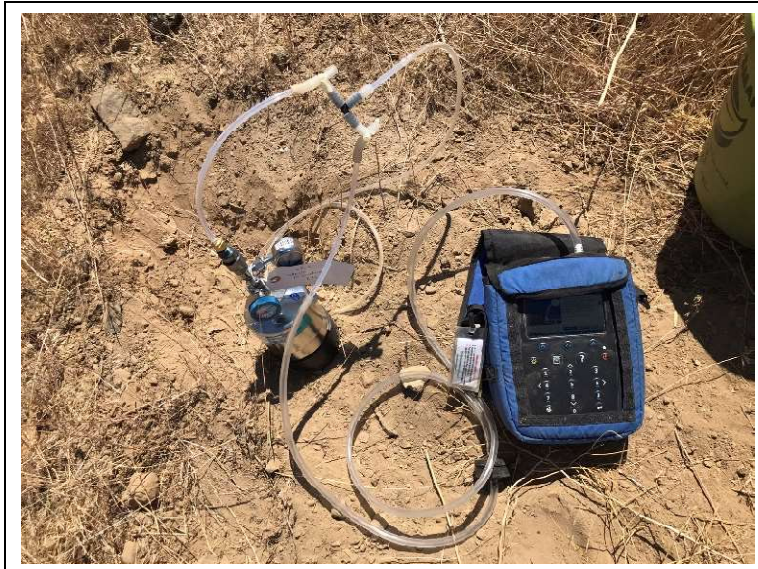
Measuring static pressure with the GEM at location VP-6
